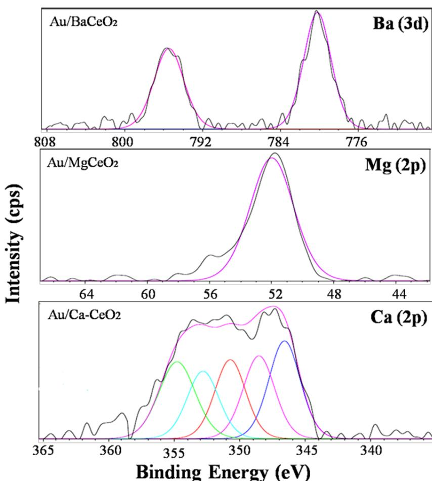
**Fig. 5:** Mg (2p), Ca (2p) and Ba (3d) core level XPS spectra.
