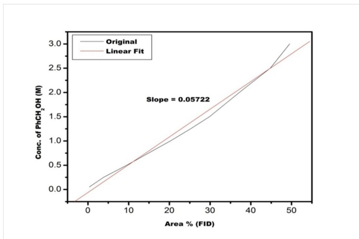
**Fig. 13: PhCH<sub>2</sub>OH Calibration**
