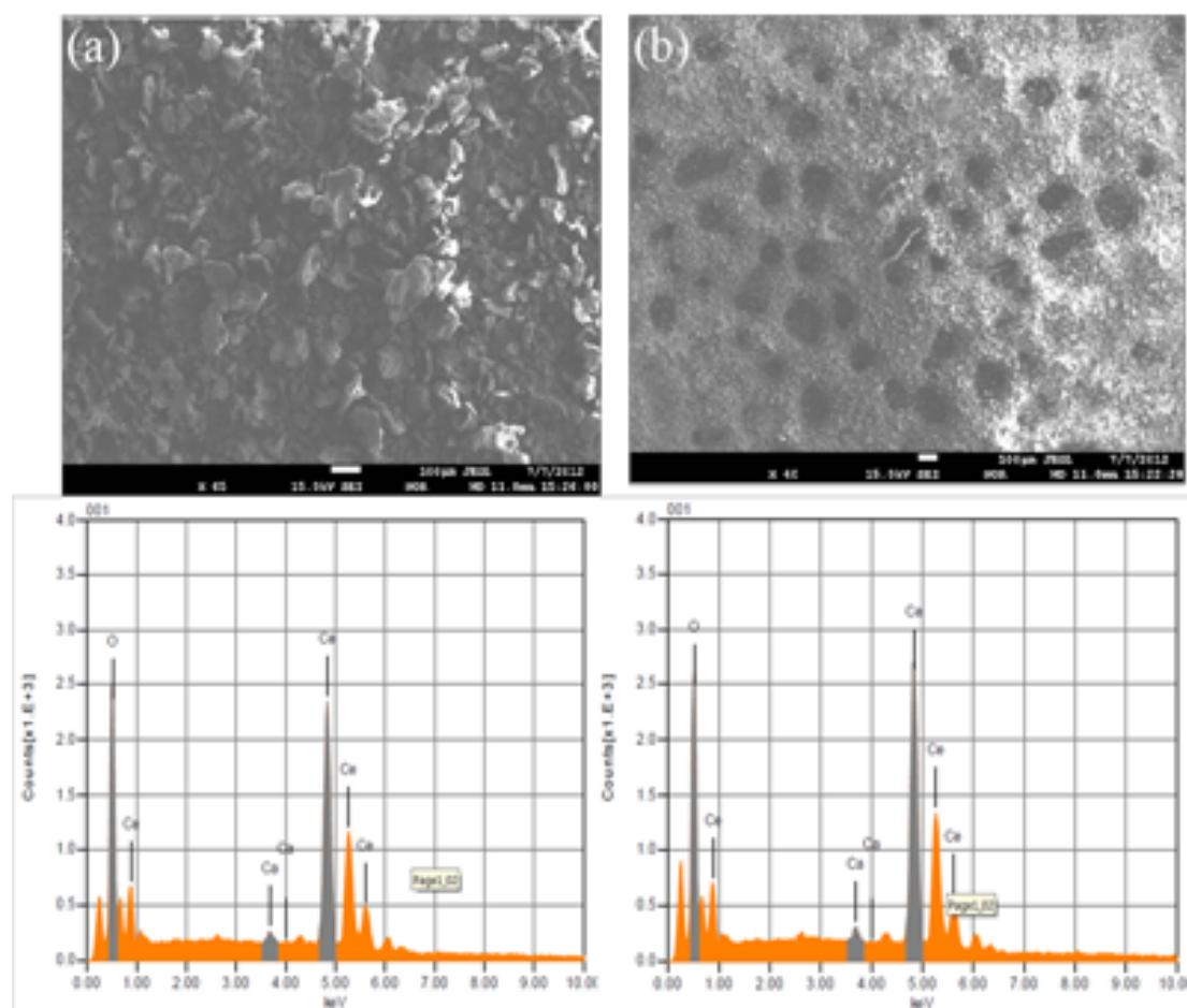
**Fig. 16: EDS analysis of Ca-CeO<sub>2</sub> ( Ca/Ce = 4/100 ) : (a) before reaction, (b) after reaction.**
