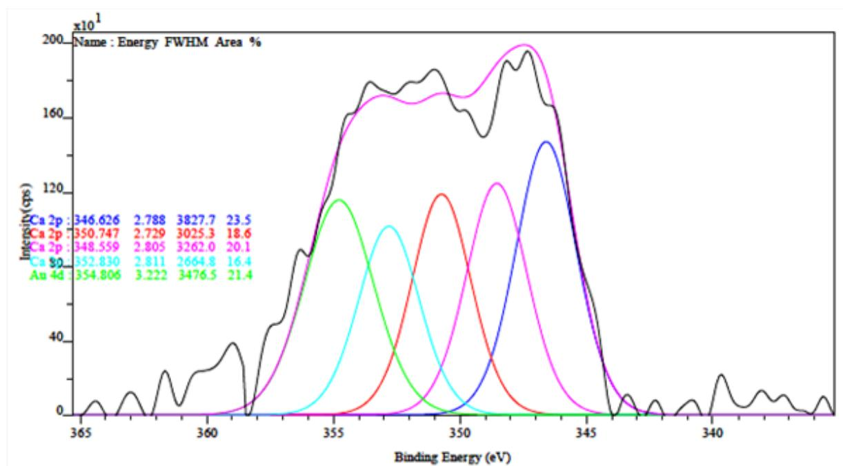
Fig. 4: Ca (2p) core level XPS spectra.
