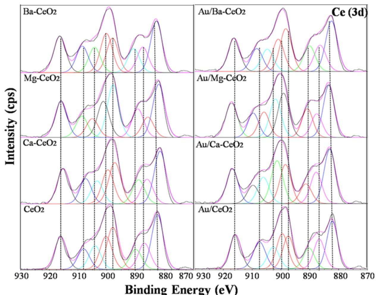
Fig. 6: Ce (3d) core level XPS spectra.
