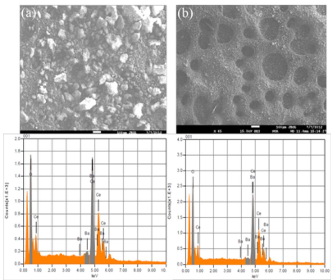
**Fig. 15: EDS analysis of Ba-CeO<sub>2</sub> ( Ba/Ce = 4/100 ) : (a) before reaction, (b) after reaction.**
