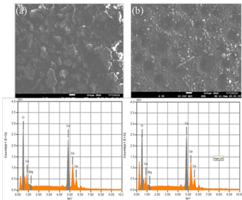
**Fig. 14: EDS analysis of Mg-CeO<sub>2</sub> ( Mg/Ce = 4/100 ) : (a) before reaction, (b) after reaction.**
