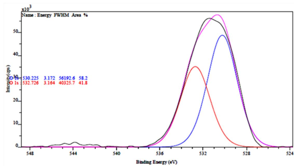
Fig. 2: O (1s) core level XPS spectra.
