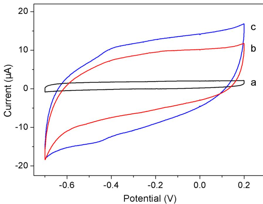
**Figure S5** CVs of bare GCE (curve a), AuNPs/rGO/GCE (curve b) and GOx/AuNPs/rGO/GCE (curve c) in N<sub>2</sub> saturated 0.2 M PBS at pH 7.4 (scan rate: 0.3 V/s).
