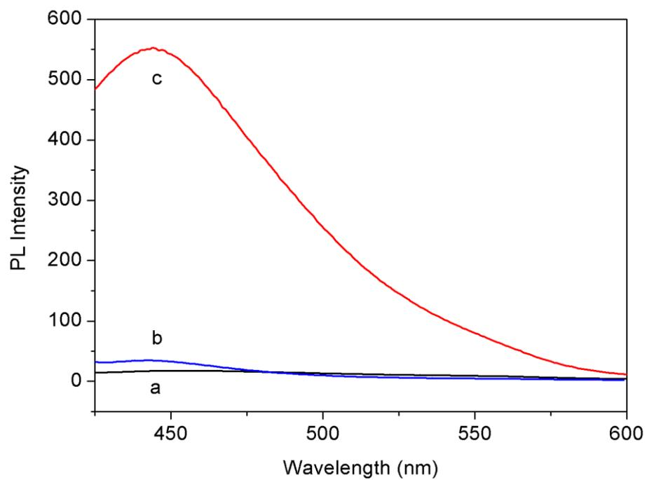
**Figure S4** PL emission spectra of aqueous dispersion of GO (curve a), CDs-GO (curve b) and CDs (curve c) (excitation at 360 nm).
