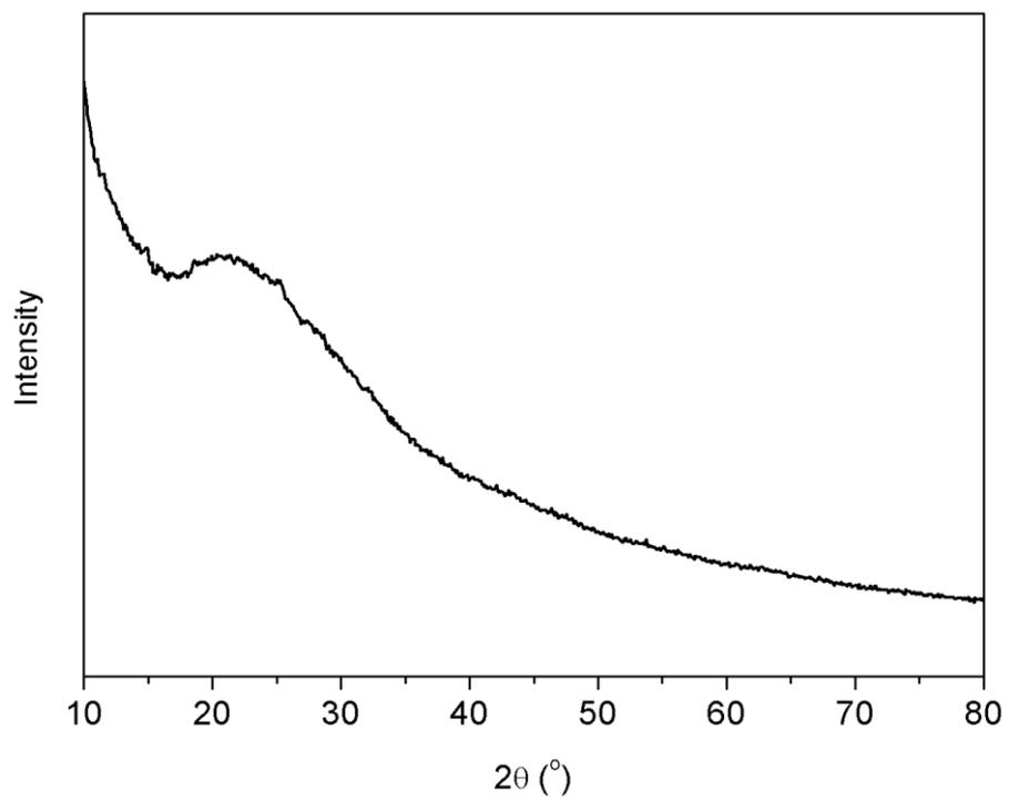
**Figure S1** The XRD pattern of the obtained CDs.
