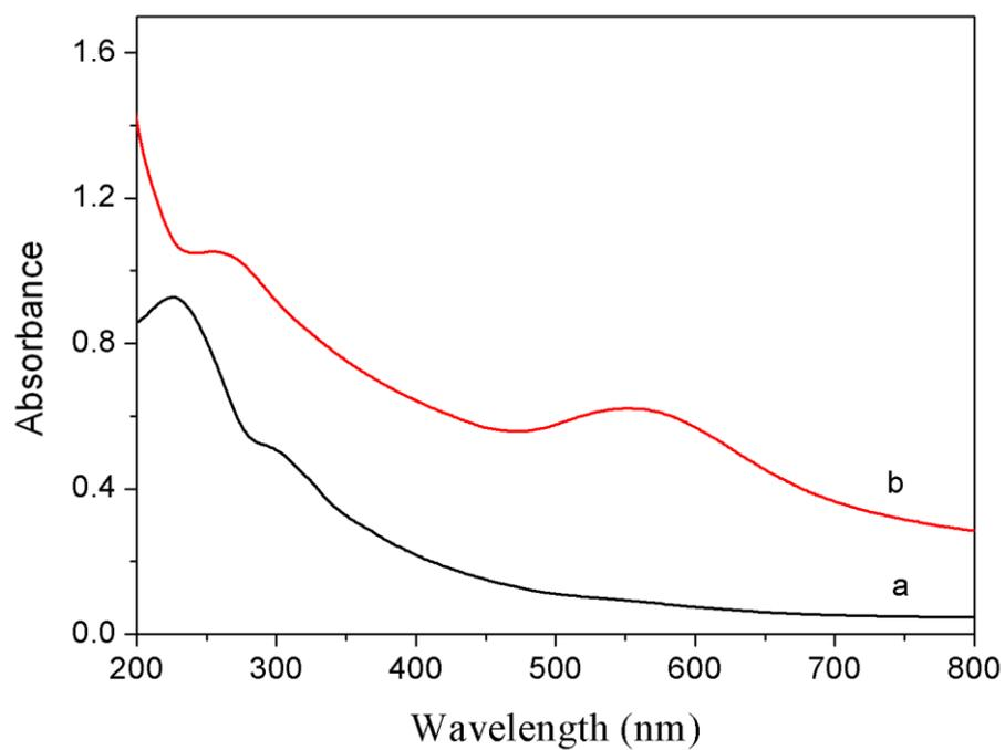
**Figure S2** UV-vis spectra of the mixture of GO and HAuCl<sub>4</sub> aqueous solution in the presence of CDs before (curve a) and after (curve b) UV irradiation.
