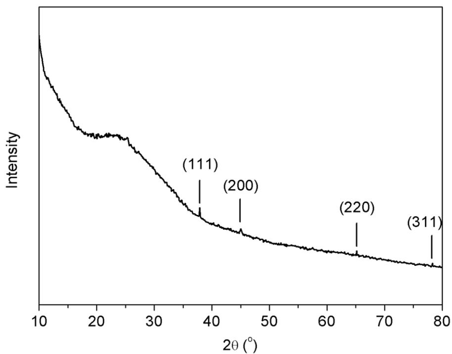
**Figure S3** The XRD pattern of the mixture of GO and HAuCl<sub>4</sub> aqueous solution in the presence of CDs after UV irradiation.
