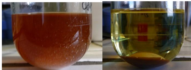
Figure 1. Oxidation of 2c with CS-S,S-5 after three runs in tert -amyl alcohol (left) and the same in hexanes after centrifugation (right).
