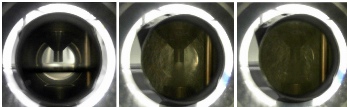
SI Figure 2 Pictures taken through the high pressure window: Liquid at the designated level (left), reaction loop pump running at 1.2 L/min (middle) and pump running at 2.1 L/min (right)
