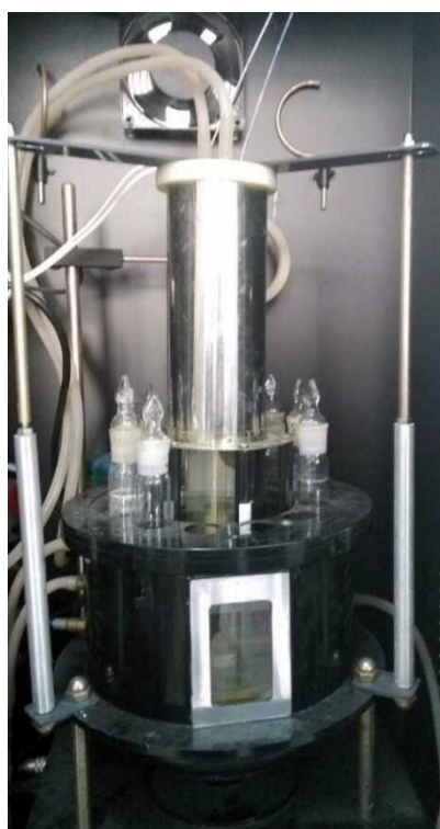
Fig. S1 Image of photocatalytic reaction equipment (XPA-7, Xujiang Electromechanical Plant, China)
