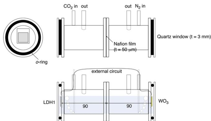
Figure S2. The design of photofuel cell-2 (larger type).
