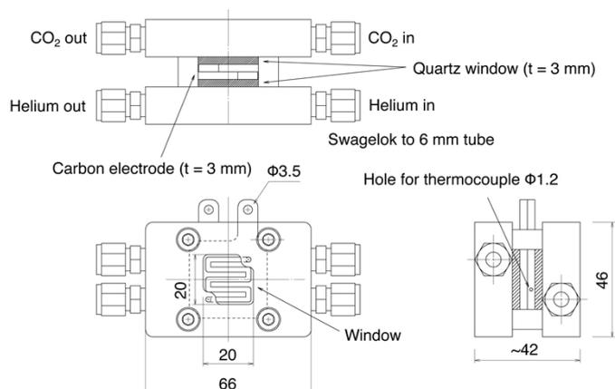
Figure S1. The design of photofuel cell-1 based on PEFC.
