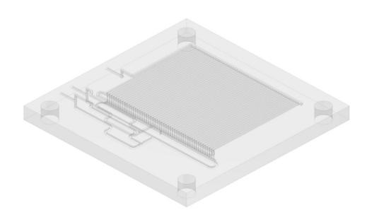
**Supporting Information Figure S1**: CAD design of the fluidic chip used in this study. For increased efficiency, both sides of the device have been machined to perform the initial droplet breakup (see main text for details) and re-joined into the main channel matrix via through holes.
