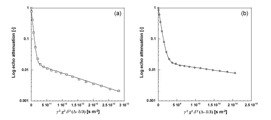
PFG-NMR attenuation plots in fresh AuPt/C plot for : (a) 1,2-propanediol and (b) water. Solid lines are fittings to Equation (1).
