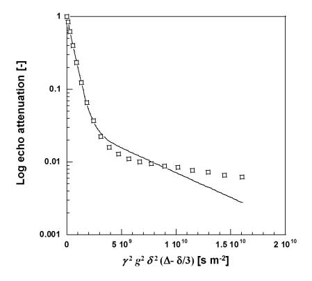
PFG-NMR attenuation data for n-octane in fresh AuPt/C fitted with a two-component diffusion model (solid line).
