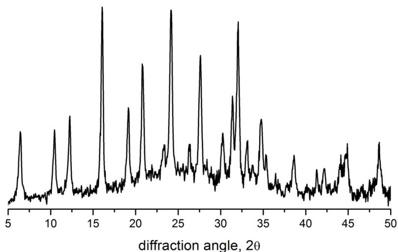
**Fig. S16.** XRD ( $\text{Cu K}\alpha$  radiation) of Cu- ZSM-5
