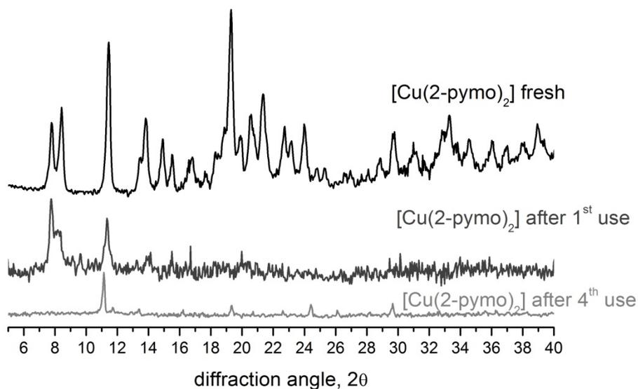
**Figure S21.** Progressive degradation of the structure of  $[\text{Cu}(2\text{-pymo})_2]$  during the oxidative coupling of 2-hydroxyacetophenone and dioxane. TGA (air flux,  $10^\circ/\text{min}$ ) of the material recovered after the first catalytic run (compare with Fig. S1).
