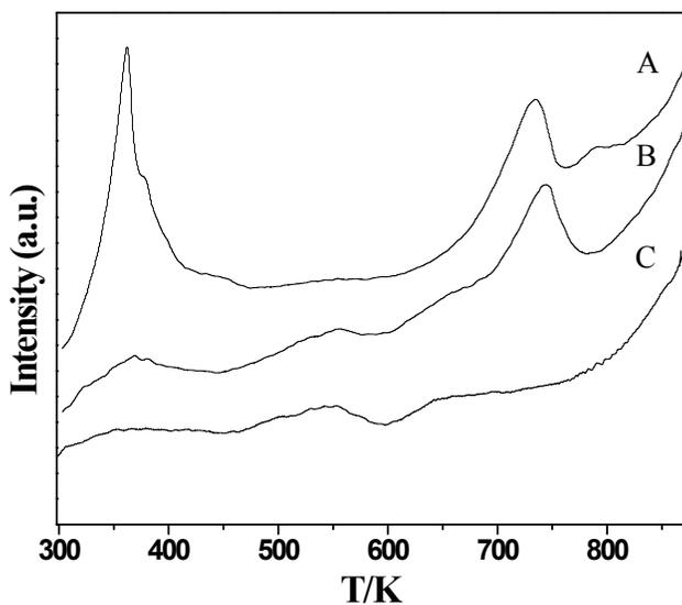
Fig. S5.  $\text{CO}_2$ -TPD profiles of the fresh and the used 25-KF/LOC-773 (A. fresh, B. the second used, C. the forth used)
