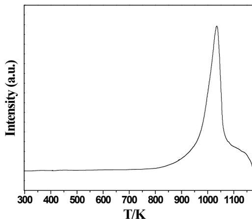
Fig. S3 TPD curve of the 25-KF/LaOC-773 catalyst without CO<sub>2</sub> pre-adsorption (blank CO<sub>2</sub>-TPD)
