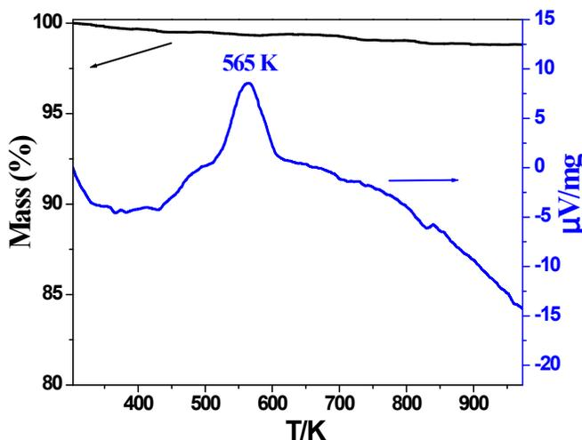
Fig. S1 the TG-DTA curves of the 25%KF/La<sub>2</sub>O<sub>2</sub>CO<sub>3</sub> precursor
