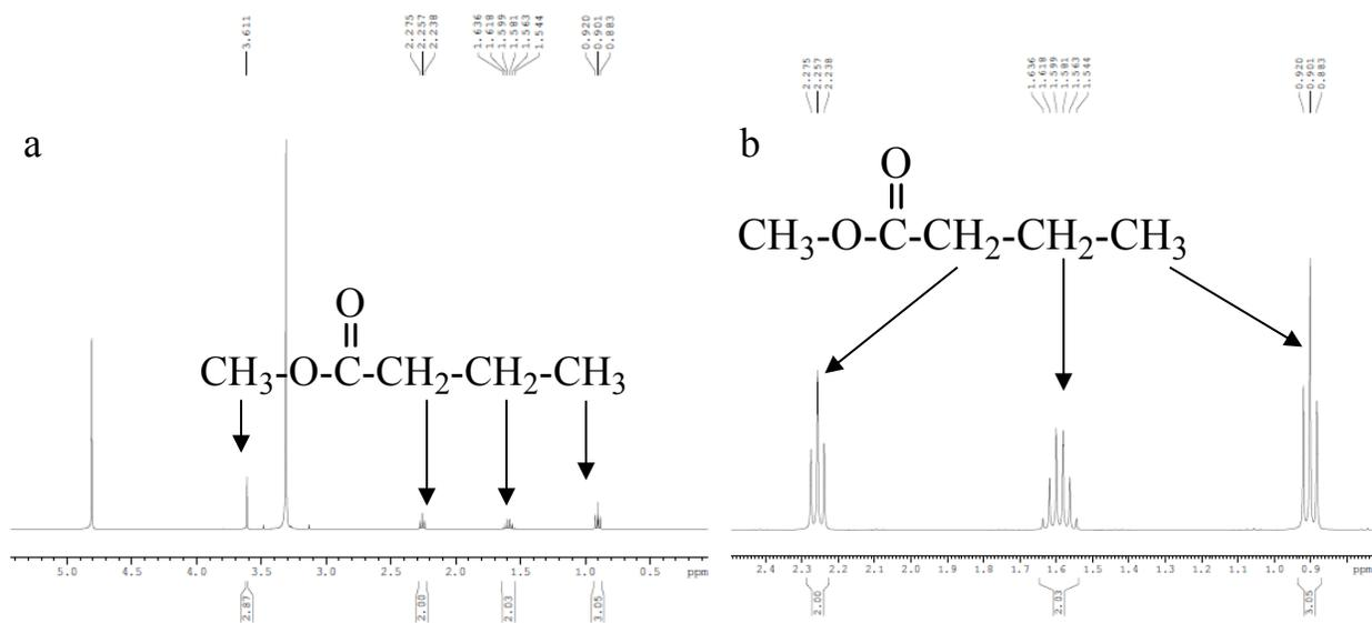
Fig. S2 <sup>1</sup>H-NMR spectra of the mixture distilled from the products of the transesterification of tributyrin with methanol at 64 °C (a. chemical shift in range of 0-5.5 ppm, b. enlarged range from 0.8 ppm to 2.5 ppm).
