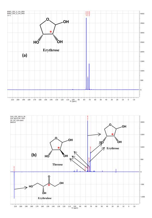
Figure S2. <sup>13</sup>C-NMR spectra of ERO a) before and b) after reaction with H-USY(6) in  $D_2O$ .
