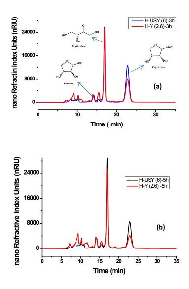
Figure S1. HPLC chromatogram of ERO reacted in water with H-Y(2.6) and H-USY(6) after a) 3 h and b) 5 h.
