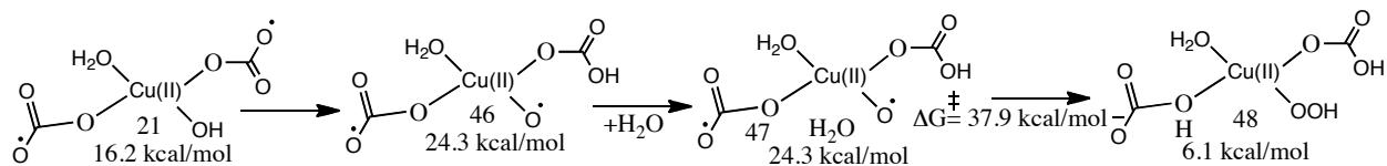
**Scheme S5.** Mechanism for the formation of a peroxy group via water nucleophilic attack on an oxo tautomer of **21**. The energies of all structures and transition states are relative to **12** at pH = 8.2.
