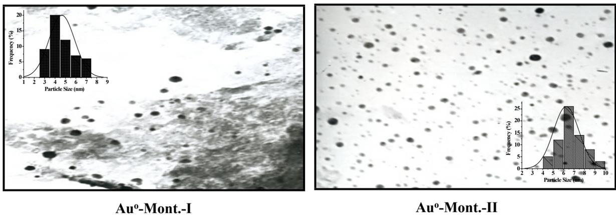
**Fig. 5:** TEM images and their corresponding particles size histogram along with a Gaussian curve fitting of Au<sup>0</sup>-Mont.-I and Au<sup>0</sup>-Mont.-II.
