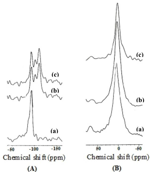
**Fig. 3.** (A)  $^{29}\text{Si}$  and (B)  $^{27}\text{Al}$  MAS-NMR spectra of (a) Parent Mont. (b) AT-Mont.-I and (c) AT-Mont.-II.
