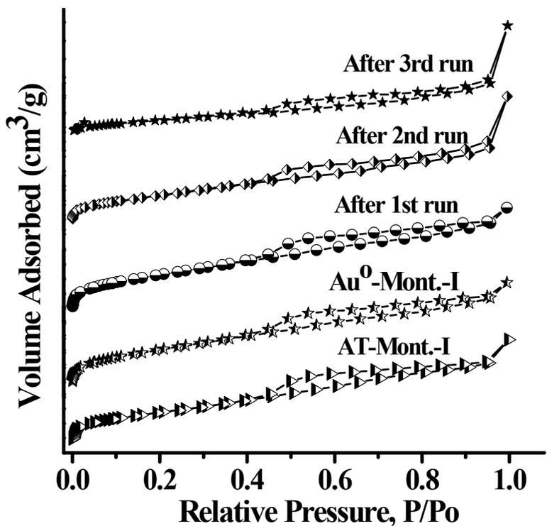
**Fig. 5.** N<sub>2</sub> adsorption / desorption isotherms of AT-Mont.-I, Au<sup>0</sup>-Mont.-I and recovered catalysts.
