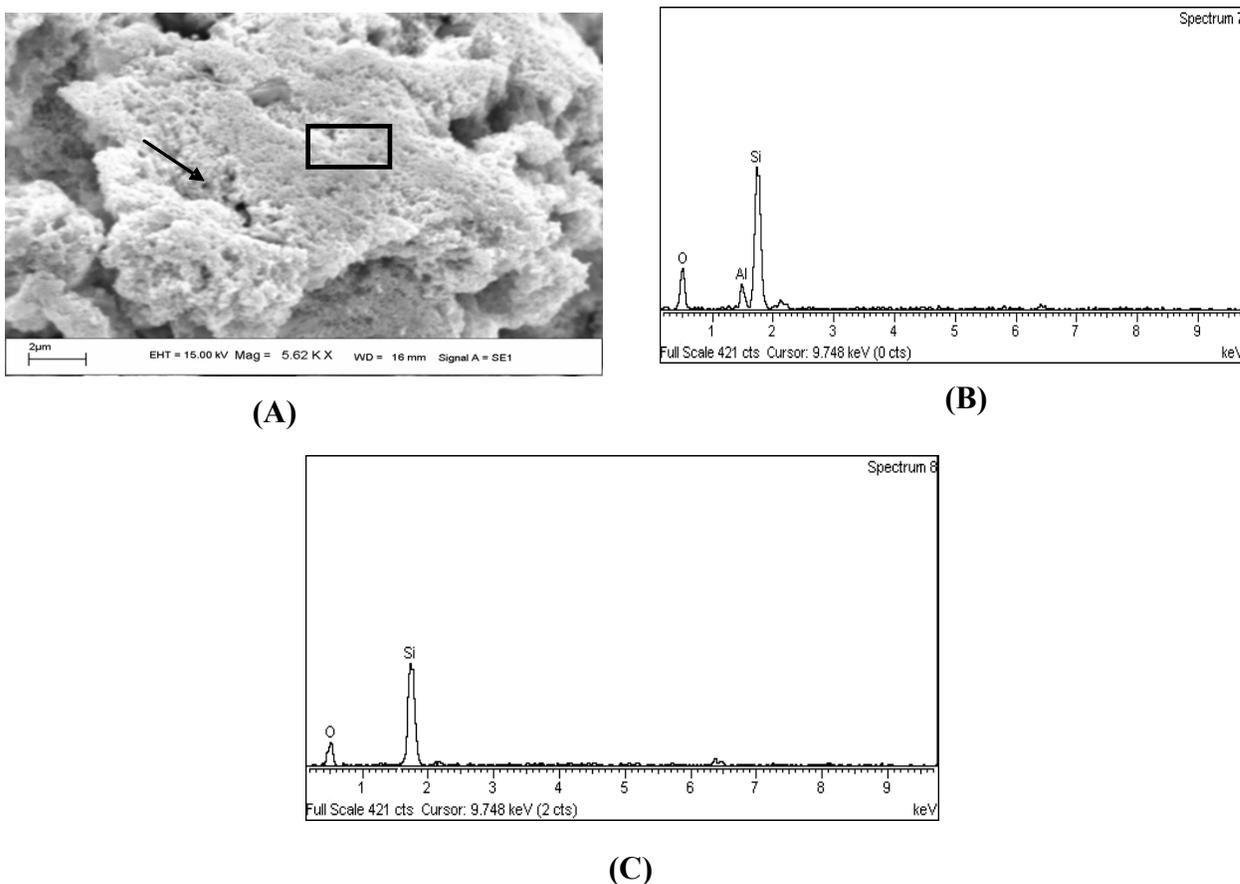
**Fig. 4.** (A) SEM image of the surface of AT-Mont.-I; (B) EDX analysis of the surface; (C) EDX spot analysis of pores (indicated by an arrow in (A)).
