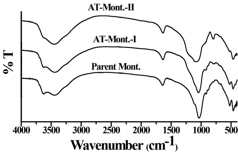
Fig. 2. FTIR spectra of different montmorillonite.
