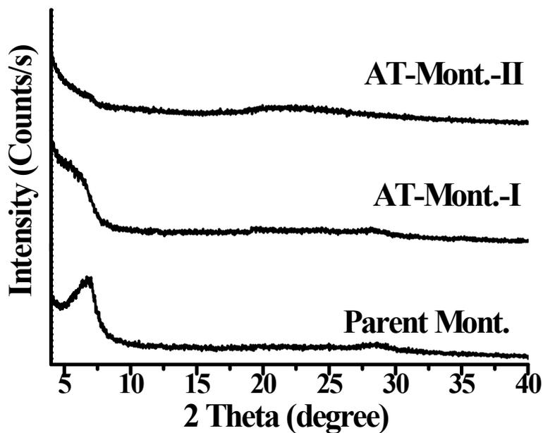
Fig. 1. Powder XRD pattern of different montmorillonite.
