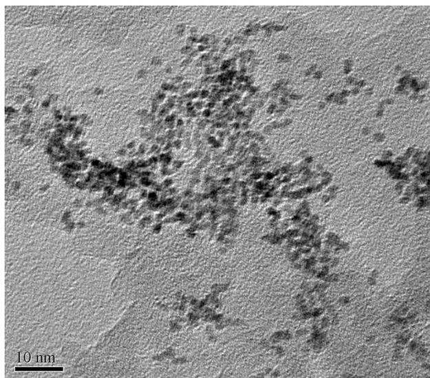
**Fig. 6.** HRTEM image of Au<sup>0</sup>-Mont.-I after 3rd run.
