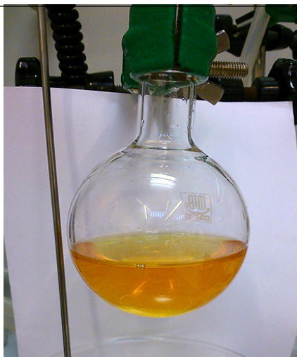
Picture S1: Reaction mixture after complete conversion of LA to GVL
