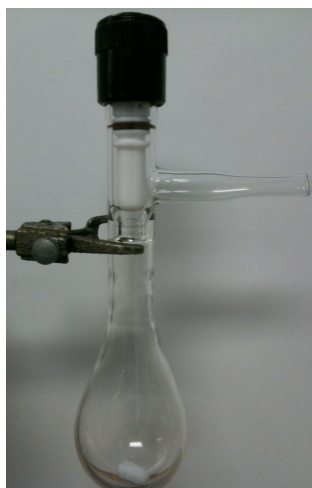
Figure S2: The Schlenk flask was prepared from a single-necked 25 mL pear-shaped flask that had its 14/20 glass joint replaced with a high vacuum threaded Teflon valve.
