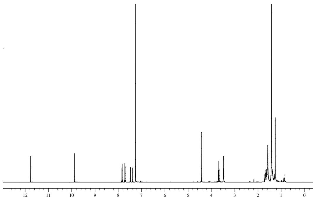
Figure S2.  $^1\text{H}$  NMR of aldehyde **3** in  $\text{CDCl}_3$
