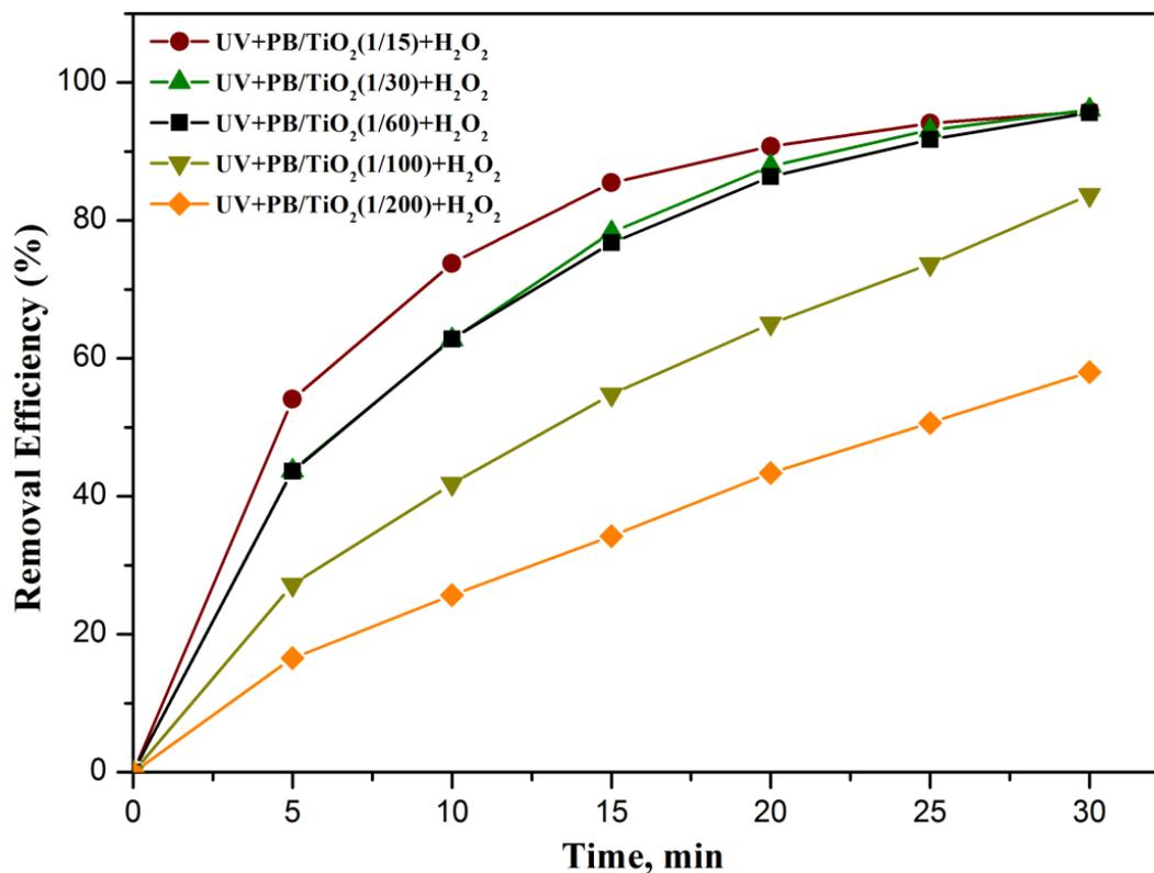
**Fig. S6.** Effect of PB content on the catalytic activities of PB/TiO<sub>2</sub> NPs for RhB degradation under UV irradiation. Reaction conditions: [RhB] = 12 mg L<sup>-1</sup>, [H<sub>2</sub>O<sub>2</sub>] = 0.4 M, catalyst = 1.0 g L<sup>-1</sup>, T = 308 K, and 27 W black light with 2.5 mW cm<sup>-2</sup> intensity.
