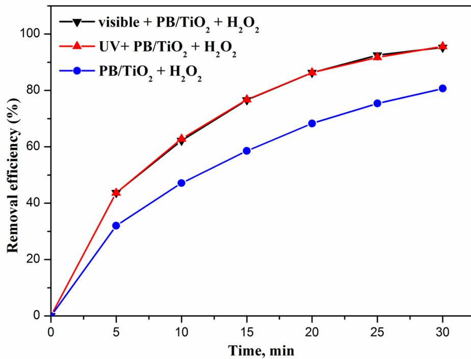
**Fig. S7.** The catalytic activities of RhB degradation in different systems. Reaction conditions: [RhB] = 12 mg L<sup>-1</sup>, [H<sub>2</sub>O<sub>2</sub>] = 0.4 M, catalyst = 1.0 g L<sup>-1</sup>, T = 308 K.
