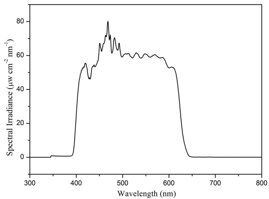
**Fig. S3.** The emission spectrum of visible light lamp used in the photo-Fenton process.
