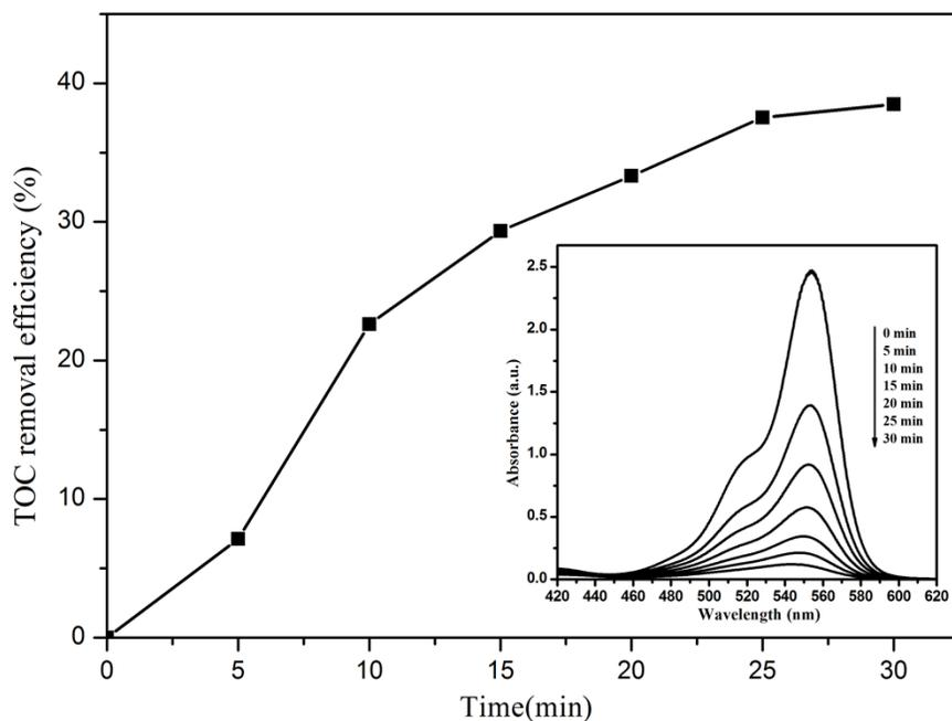
**Fig. S4.** The TOC removal efficiency of RhB in the photo-Fenton process. (Inset: The UV-vis absorption spectra of RhB during the photo-Fenton process at different time intervals.) Reaction conditions:  $[\text{RhB}] = 12 \text{ mg L}^{-1}$ ,  $[\text{H}_2\text{O}_2] = 0.4 \text{ M}$ , catalyst =  $1.0 \text{ g L}^{-1}$ , and  $T = 308 \text{ K}$ .
