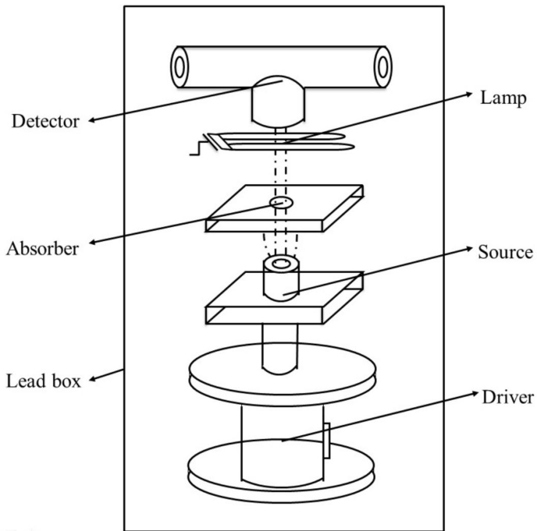
**Fig. S1.** Diagram of room temperature  $^{57}\text{Fe}$  Mössbauer measurement setup with UV lamp in this study.
