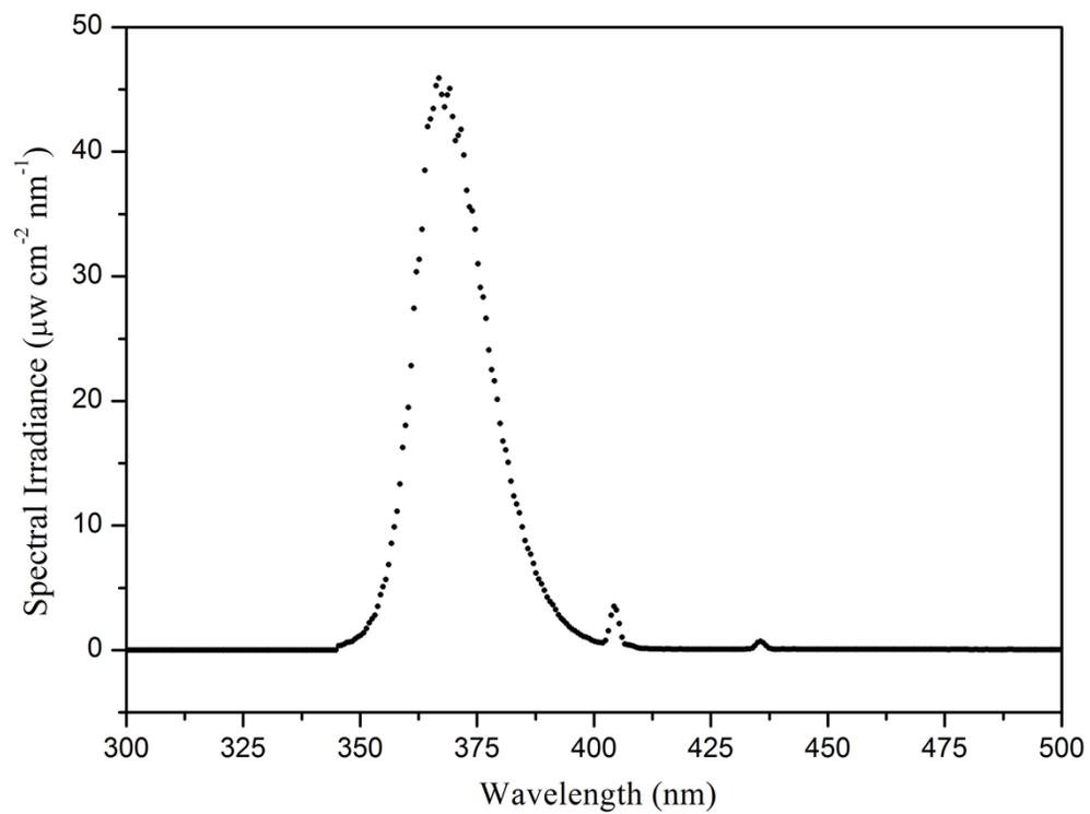
**Fig. S2.** The emission spectrum of UV lamp used in the photo-Fenton process.
