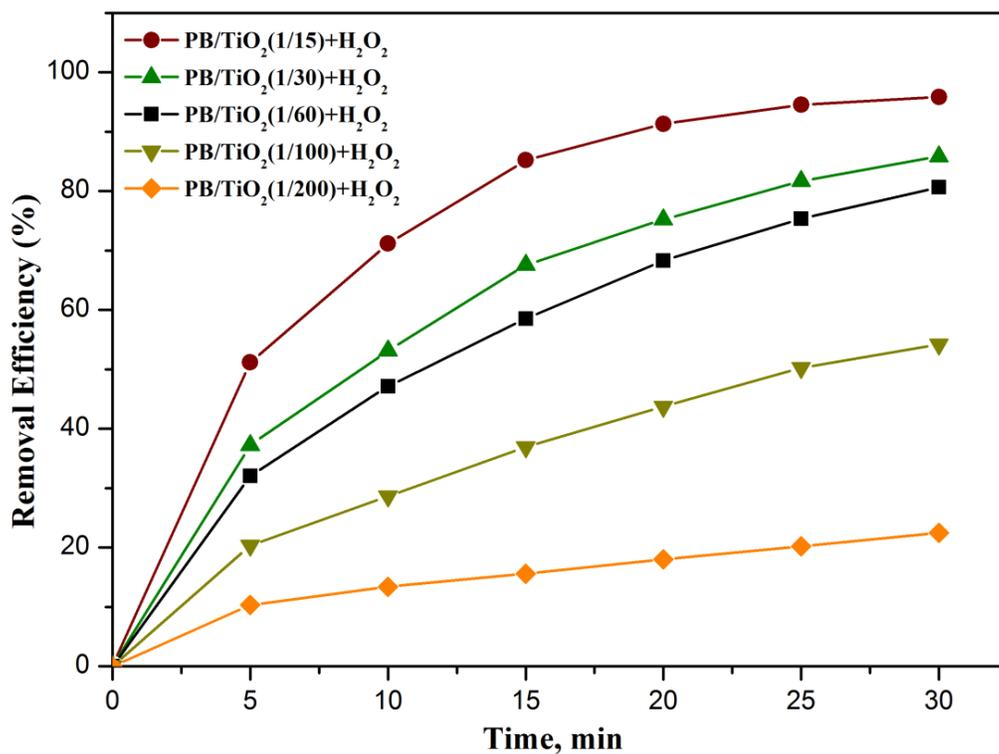
**Fig. S5.** Effect of PB content on the catalytic activities of PB/TiO<sub>2</sub> NPs for RhB degradation in dark. Reaction conditions: [RhB] = 12 mg L<sup>-1</sup>, [H<sub>2</sub>O<sub>2</sub>] = 0.4 M, catalyst = 1.0 g L<sup>-1</sup>, and T = 308 K.
