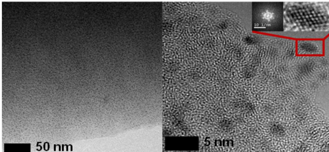
Fig. 2: TEM analysis of the Ir@SiCN catalyst. left: overview; right: HR-TEM.
