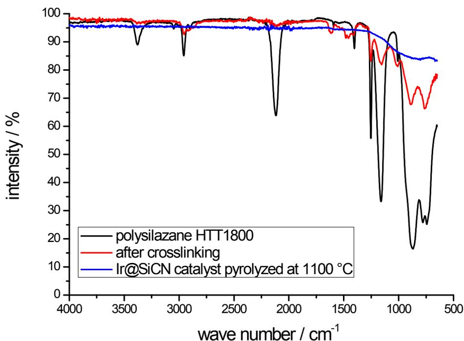
Fig. 1: FT-IR study of the Ir@SiCN nano composite synthesis
