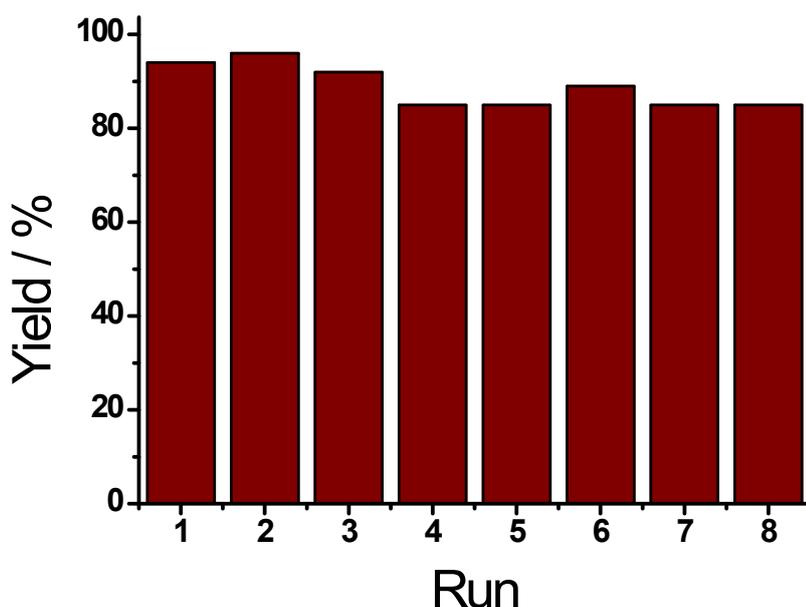
Fig. 5: Reusability of the Ir@SiCN catalyst; the catalyst was recovered after each run
