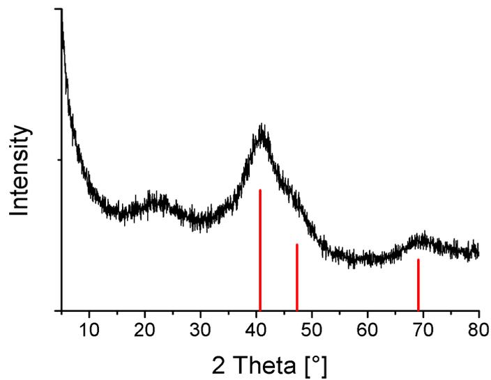
Fig. 3: Powder XRD analysis of the Ir@SiCN catalyst (red: Reflexes of cubic crystalline iridium; reference card: 00-046-1044)
