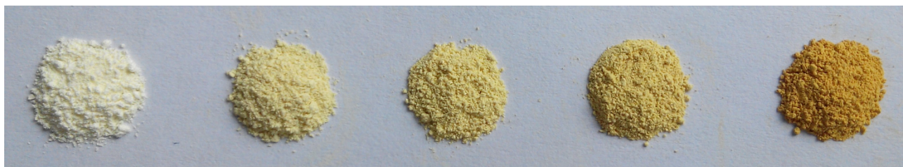
Fig. S1 \text{CeO}_2 , \text{Ce}_{0.95}\text{Bi}_{0.05}\text{O}_{2-\delta} , \text{Ce}_{0.9}\text{Bi}_{0.1}\text{O}_{2-\delta} , \text{Ce}_{0.8}\text{Bi}_{0.2}\text{O}_{2-\delta} and \text{Ce}_{0.5}\text{Bi}_{0.5}\text{O}_{2-\delta} powder from left to right.
