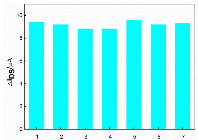
**Fig. S7.** The repeatability of the proposed sensor for the detection of target GAA TNR (10pM).
