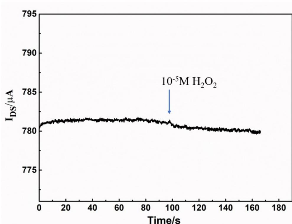
**Fig. S2.** The channel current response after adding  $10^{-5} H_2O_2$  to the electrolyte. (Ag/AgCl reference electrode is used as the gate electrode)
