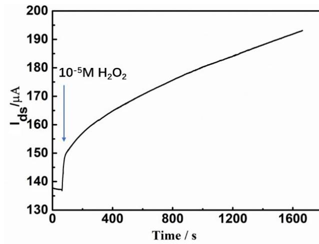
**Fig. S3.** The channel current responses of sensor to the addition of  $\text{H}_2\text{O}_2$  at the operational voltages of  $V_G = 0.6 \text{ V}$  and  $V_{DS} = 0.05 \text{ V}$  on the broken graphene.
