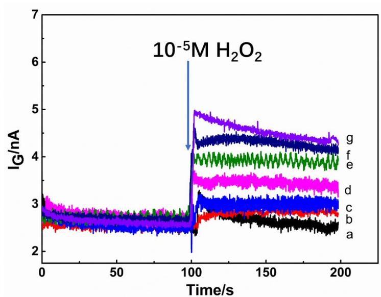
**Fig. S5.** Gate current of the SGGT during the additions of GAA TNR with different concentrations ((a) 0.1 pM; (b) 1 pM; (c) 10 pM; (d) 100 pM; (e) 1 nM; (f) 10 nM; (g) 100 nM).
