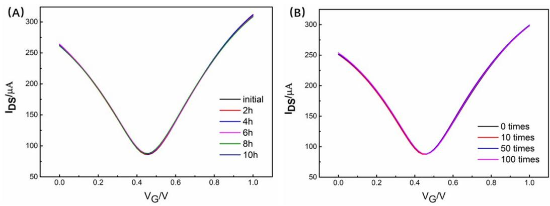
**Fig. S8.** The transfer characteristics of SGGT measured in PBS solution (A) from initial to 10h. (B) from 0 times up to 100 times.
