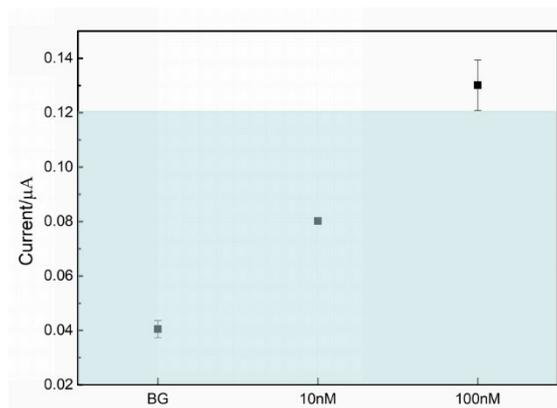
**Fig. S6.** A scatter plot of different concentrations of target DNA when DNAzyme-modified gate electrode was used as work electrode in traditional three-electrode electrochemical platform. The blue region indicates that a signal to noise ratio are less than 3. The number of test samples for each set of data is 3.
