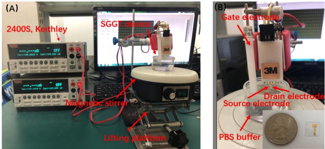
**Fig. S1.** (A) Actual test photo of the device. (B) structure photo of the device. Inserted image displayed that the real size of the chip compared with Quarter Dollar.
