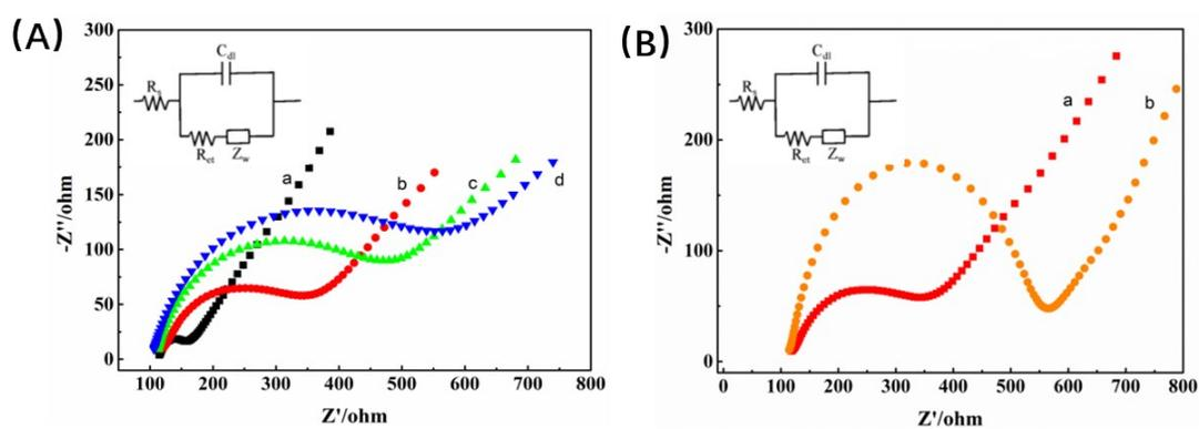
**Fig. S4.** (A) EIS (potential of 0.175 V, frequency range of 0.1 Hz to 100 kHz, alternating potential of 5 mV) of for the progressively modified gate electrodes, the points correspond to the (a)bare GCE (b)CHIT-SA/PANI/GCE (c)Bio-DNA/CHIT-SA/PANI/GCE(M-gate) (d)Hemin/Rep-DNA/T-DNA/M-gate.(T-DNA,100pM). (B) Nyquist plots of (a) CHIT-SA/PANI/GCE (b) CHIT-SA/GCE.
