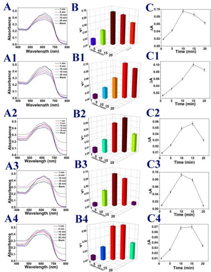
**Fig. S3** (A-A4) UV-vis spectra of EBT (2  $\mu$ M)-QA (100 nM)-lanthanide ion (10 nM) solutions at different incubation time. (B-B4,C-C4) Change of absorbance of EBT at 615 nm at different incubation time. (A,B,C) La<sup>3+</sup>, (A1,B1,C1) Sm<sup>3+</sup>, (A2,B2,C2) Eu<sup>3+</sup>, (A3,B3,C3) Gd<sup>3+</sup>, (A4,B4,C4) Yb<sup>3+</sup>.
