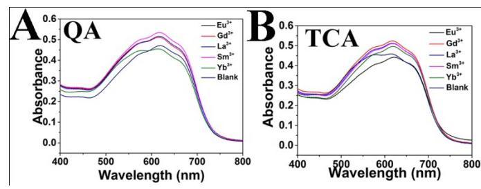
**Fig. S5** The UV-vis absorption spectra of (A) QA, and (B) TCA before and after addition of different lanthanide ions at 10 nM.
