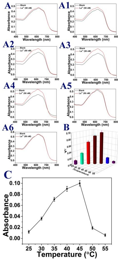
**Fig. S2** UV-vis spectra of EBT (2  $\mu$ M)-QA (100 nM)-La<sup>3+</sup> (10 nM) solutions at different temperatures. (A) 25 °C, (A1) 30 °C, (A2) 35 °C, (A3) 40 °C, (A4) 45 °C, (A5) 50 °C, (A6) 55 °C. (B,C) Change of absorbance of EBT at 615 nm at different temperatures.
