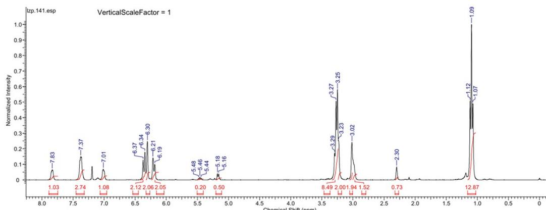
Fig. S1. <sup>1</sup>H NMR spectrum of compound **RBA**.
