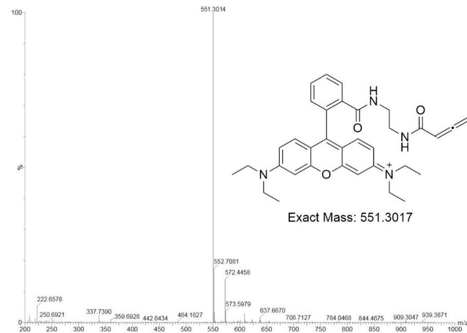
**Fig. S3.** ESI-HRMS spectrum of probe RBA.
