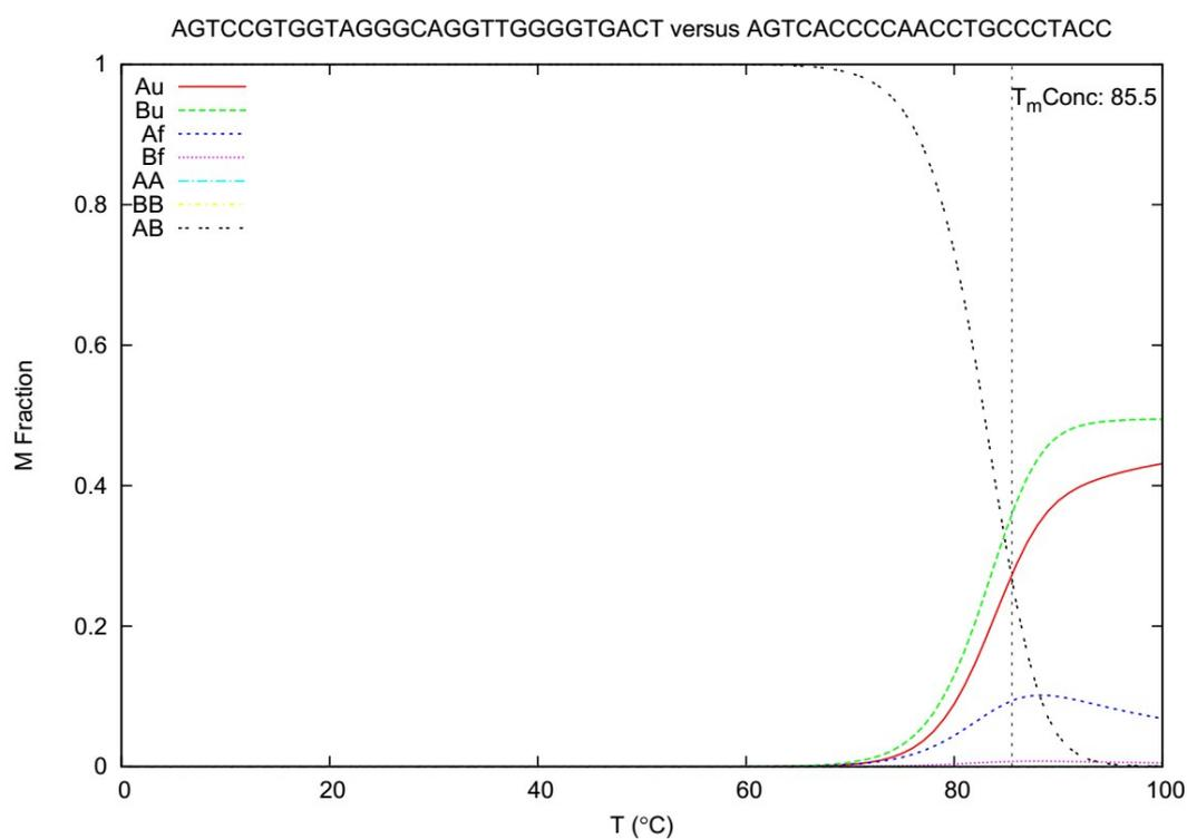
Fig. S2 Mole fractions of aptamer (A) and catalyst (B) are computed as a function of temperature by UNAFold. Au represents unfolded aptamer; Af represent folded aptamer and AA represent homodimer. The mole fractions of different molecular species were computed using the computed free energies for individual monomer (folded) and dimer (hybridized) species.
