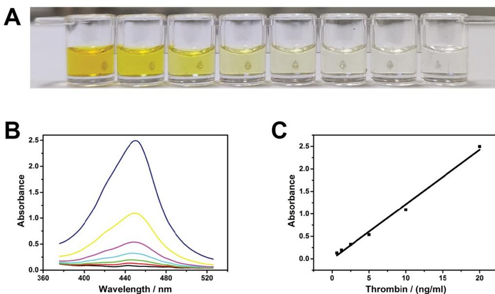
Fig. S6 (A) Photographs of ELISA results for thrombin detection with the bare eyes. (B) Corresponding plasmon absorption spectra for different thrombin concentrations. (C) the liner range (0.625 to 20 ng/mL.) between the absorption intensity at 450 nm and thrombin.
