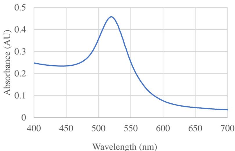
**Fig. S1** UV-Vis spectrum of synthesized 20nm AuNPs. The  $\lambda_{\text{LSPR}}$  was measured to be 520nm.
