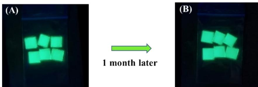
**Fig. S7.** Photographs of PDMS film and PDMS film placed in sealable bag for 1 month.(under 302nm UV light)
