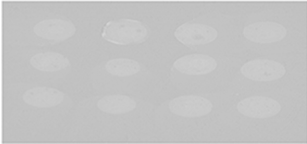
Fig. S1 differential SPRi image obtained on conventional gold chip after 20 min reaction with 100 µg mL -1 OTA antibody solution.
