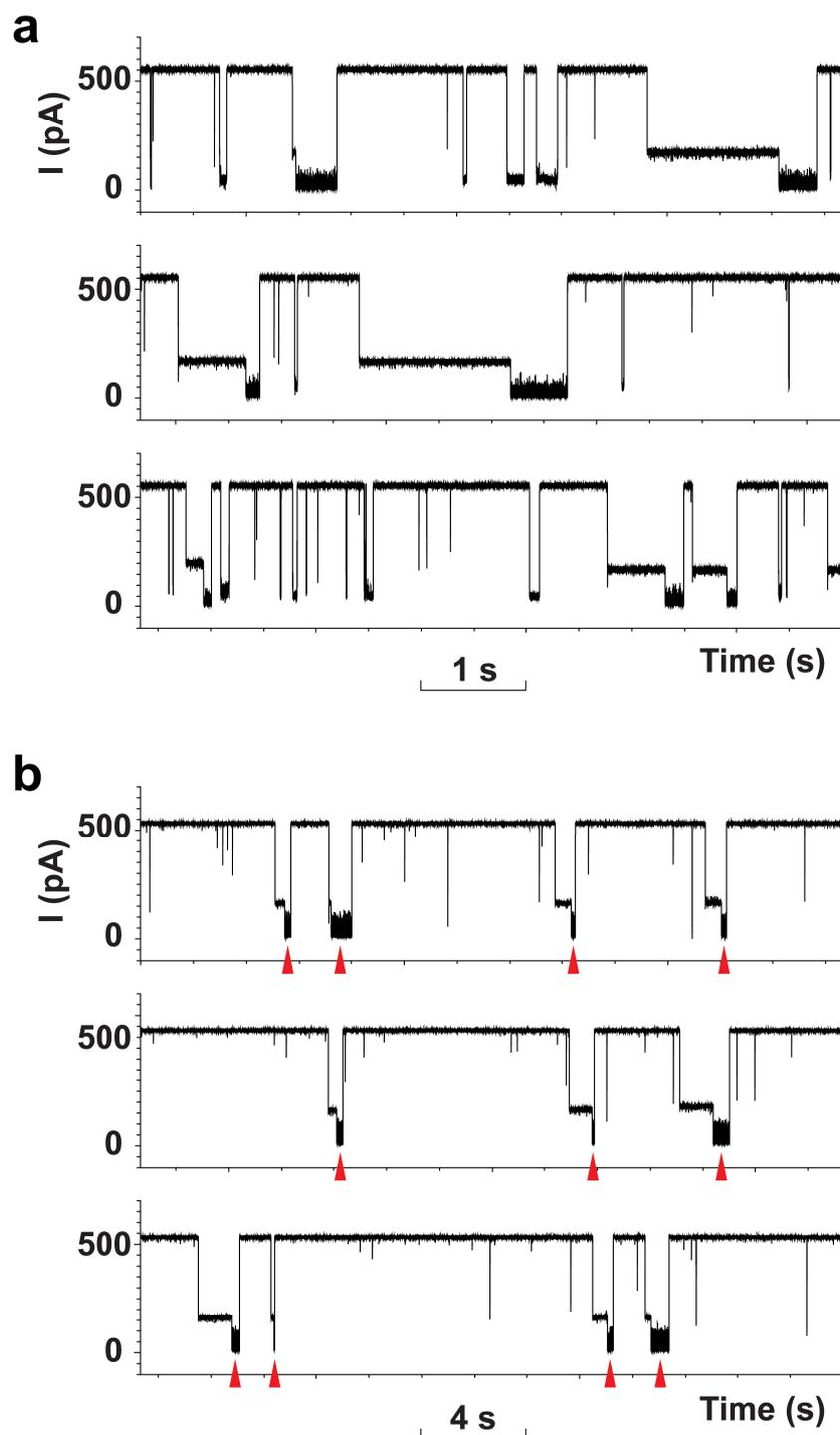
**Figure S5.** Comparison of the current traces before and after removal of duplex DNA in microRNA sensing with tMB probe. **(a)** There were many unwanted current events in the trace before the duplexes were removed. **(b)** After using magnetic beads, the trace became very clean. The red arrows indicate current signatures. All data were acquired in the buffer of 3 M KCl, 10 mM MES and 10 mM MgCl<sub>2</sub>, pH 8.0, with the transmembrane potential held at +200 mV.
