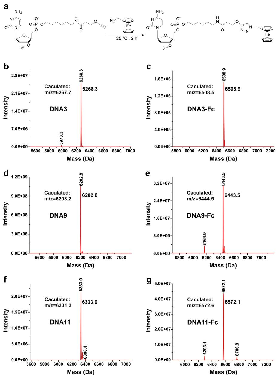
**Fig. S1** Modification of DNA1, DNA3, DNA5 and mass spectroscopic characterization. (a) Chemical modification of DNA1, DNA3, DNA5 with azidomethylferrocene via “click” chemistry. Mass spectroscopic characterization of DNA3 (b); DNA3-Fc (c); DNA9 (d); DNA9-Fc (e); DNA11 (f); DNA11-Fc (g).
