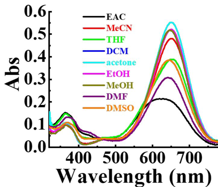
**Fig. S5** Absorption of L1 (10.0  $\mu\text{M}$ ) in different solvents. Ethyl acetate (EAC), acetonitrile (MeCN), tetrahydrofuran (THF), dichloromethane (DCM), ethanol (EtOH), methanol (MeOH), N, N-dimethylformamide (DMF), dimethyl sulfoxide (DMSO).
