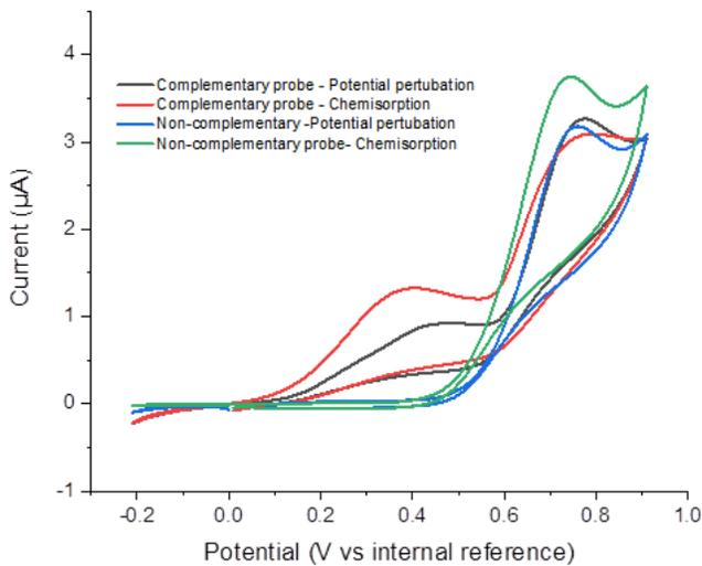
Figure S7: Cyclic voltammograms of the ssDNA modified electrodes after the DNA-detection step recorded in measuring buffer (50 mM Tris. HCl, 10 mM MgCl<sub>2</sub>, pH 9.6) containing 3 mM pAPP. Scan rate, 0.1 V/s. Current vs in-built reference electrode potentials are presented here
