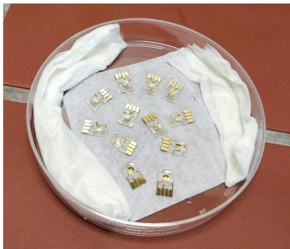
Figure S4: Microelectrodes kept in humid conditions with wet tissue papers in the vicinity and sealed for overnight immobilization of ssDNA through chemisorption.
