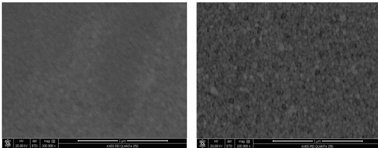
Figure S1. Scanning electron microscopy (SEM) images of the gold-sputtered electrodes after cleaning in an ultrasonic bath with 70% ethanol and water (Protocol 2) and after additional electrochemical pretreatment (Protocol 5).
