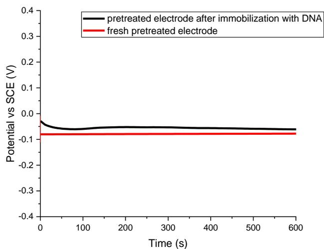
Figure S5: Open circuit potential between SCE and gold built-in reference electrode from freshly pretreated (protocol 5) bare microelectrode and pretreated (protocol 5) microelectrode after DNA/MH modification.
