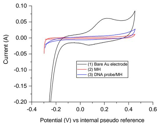
Figure S2. Evaluation of the potential window of the electrodes in the immobilization buffer used for the potential pulse assisted immobilization: (1) a bare gold-sputtered electrode, (2) an electrode coated with 1 mM
