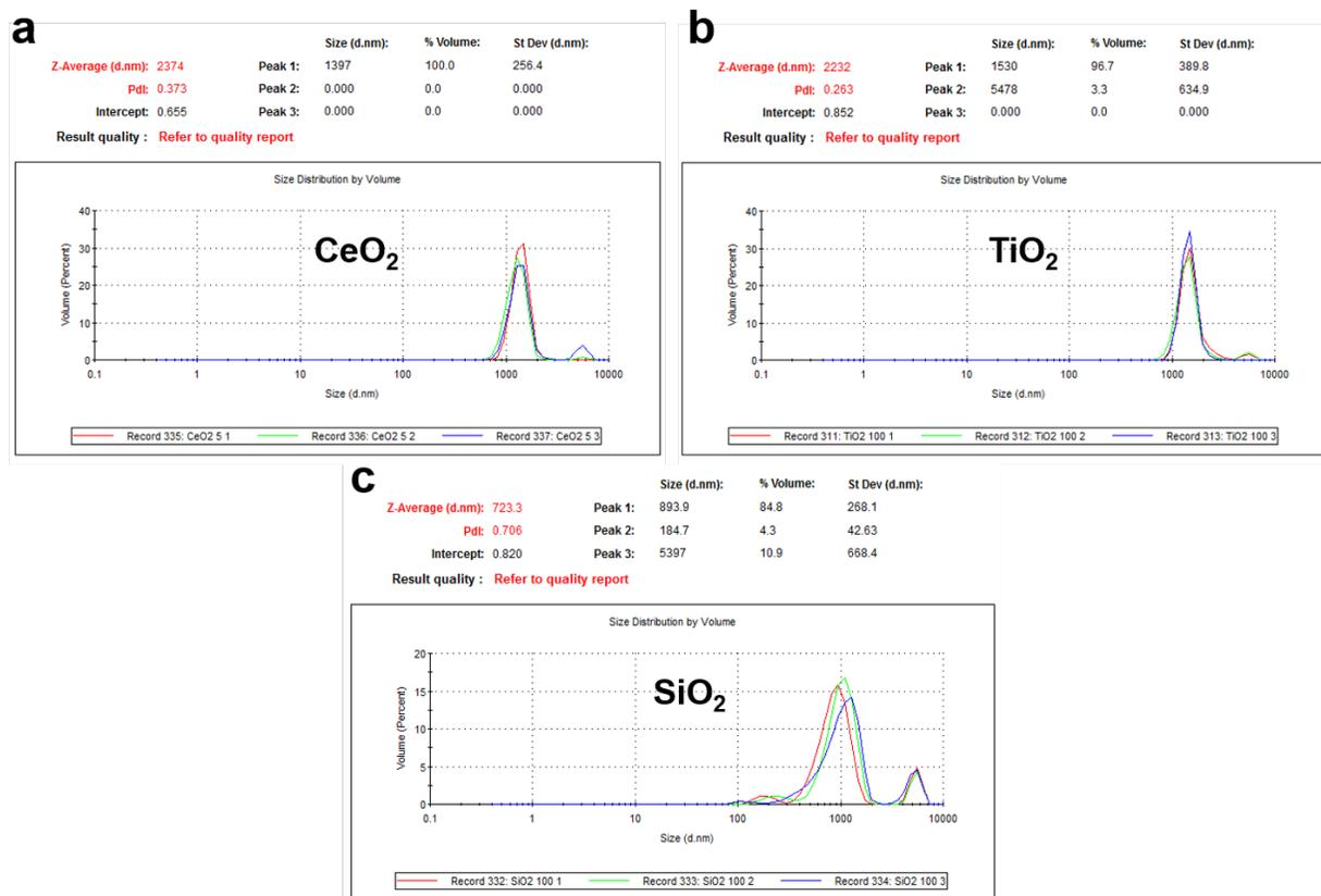
**Figure S2** DLS-based hydrodynamic size determination using Zeta-Sizer on (a) CeO<sub>2</sub>, (b) TiO<sub>2</sub> and (c) SiO<sub>2</sub> NPs at 100 µg/mL original dosage in pH 7.4 serum-free culture medium F-12K. Large agglomerates with sizes that peaked at 1397 nm in CeO<sub>2</sub> NPs, and at 1530 nm and 5478 nm in TiO<sub>2</sub> NPs were observed, while relatively smaller agglomerates with sizes that peaked at 893.9 nm and 184.7 nm were observed in SiO<sub>2</sub> NPs.
