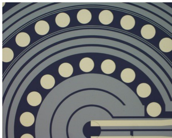
Figure S3. Borofloat glass bottom substrate with heaters shown in gray and Au layer at the bases of the pillars and fluidic port where eutectic bonds will occur in white.
