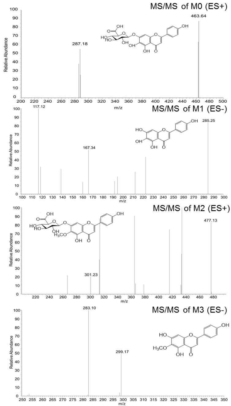
**Figure S2.** MS/MS spectra of scutellarin and its metabolites (M0-M3) in both positive and negative ion mode.<sup>1-3</sup>
