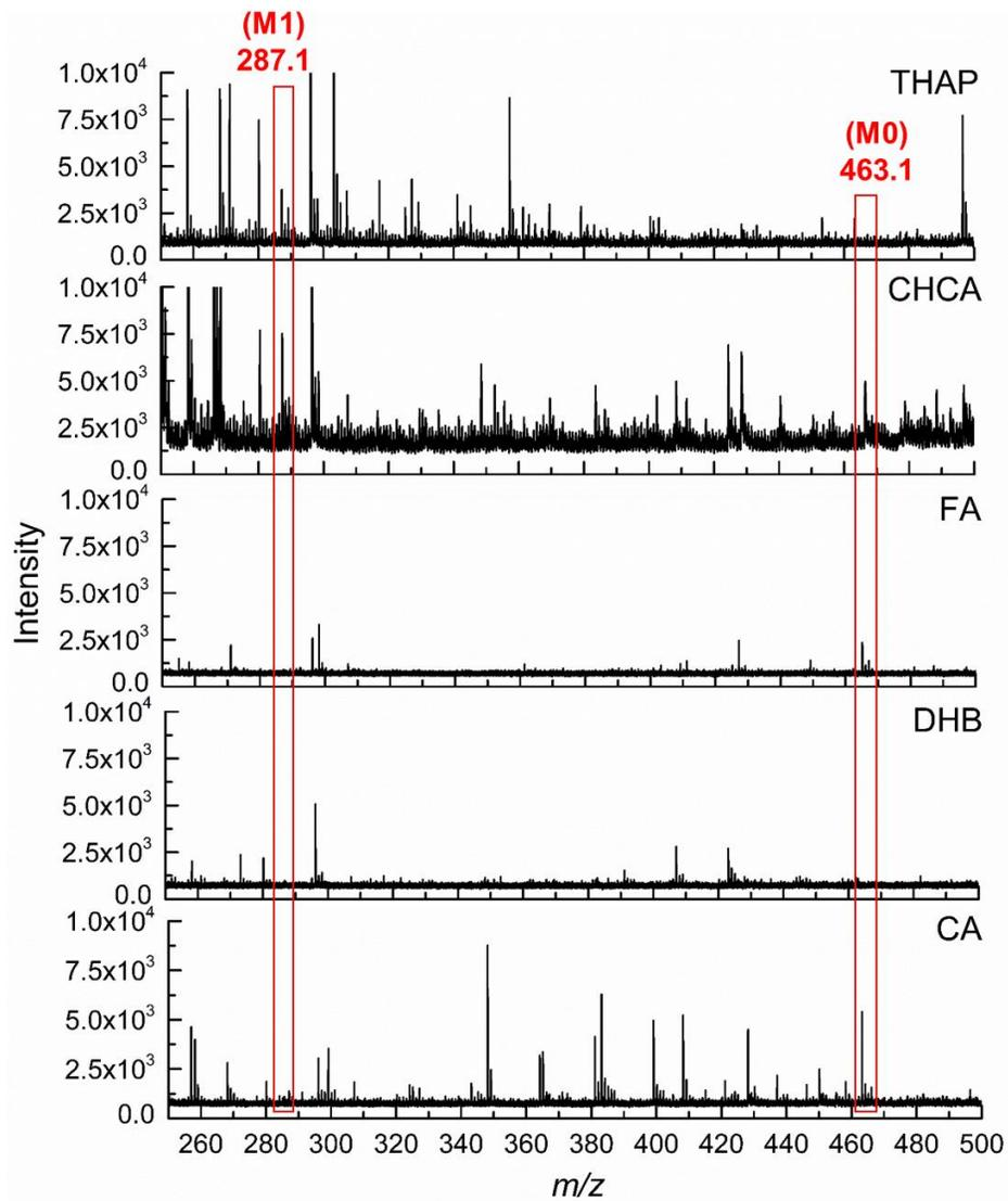
**Figure S4.** The MALDI mass spectra of scutellarin ( $m/z$  463.1) and its metabolites ( $m/z$  287.1,  $m/z$  477.1,  $m/z$  301.0) with THAP, CHCA, FA, DHB and CA matrix in the positive ion mode. The matrix was deposited on scutellarin-treated kidney tissue sections.
