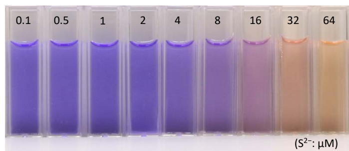
Fig. S10. Color changed of PAPS-Pd (10 \mu\text{M} ) in the presence of different concentrations of \text{S}^{2-} in pH 10.2 carbonate buffer.
