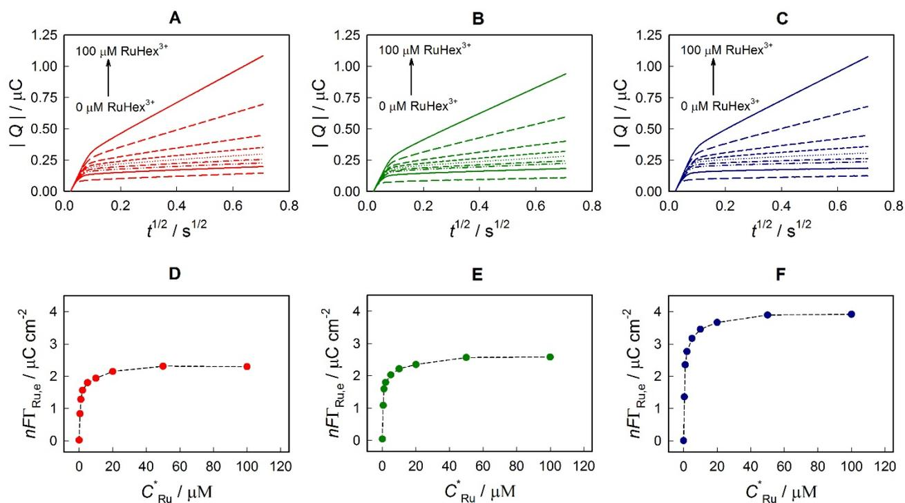
**Figure S8.** (A-C) Chronocoulometric curves, and (D-F) the corresponding adsorption isotherms obtained for the probe DNA-modified electrodes recorded in 10 mM Tris buffer (pH 7.4) containing different concentrations of  $\text{RuHex}^{3+}$ .  $\Gamma_{\text{DNA}}$  is (A and D) 1.17, (B and E) 1.90, and (C and F) 3.24  $\text{pmol cm}^{-2}$ . Dashed lines in D-F are given as a guide to the eye only.
