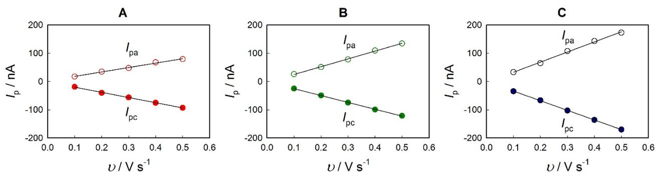
**Figure S2.** Plots of the CV peak currents versus  $\nu$  for the electrodes modified with different amounts of the probe DNA and MB-labeled cDNA (with MB attached to the 5'-end). The DNA surface coverage was (A) 1.17, (B) 1.90, and (C) 3.24  $\text{pmol cm}^{-2}$ . Voltammograms were recorded in 10 mM Tris buffer (pH 7.4) / 0.15 M NaCl.
