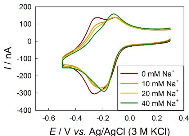
**Figure S7.** CV curves of a probe DNA-modified electrode recorded in 10 mM Tris buffer (pH 7.4) containing 20  $\mu\text{M}$   $\text{RuHex}^{3+}$  and different concentrations of  $\text{Na}^+$  cation ( $v = 0.1 \text{ V s}^{-1}$ ).
