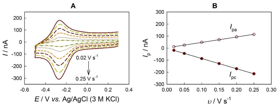
**Figure S6.** (A) CV curves at different  $v$ , and (B) the corresponding plot of the peak currents versus  $v$  for a probe DNA-modified gold electrode. Measurements were performed in 10 mM Tris buffer (pH 7.4) containing  $2 \mu\text{M RuHex}^{3+}$ .
