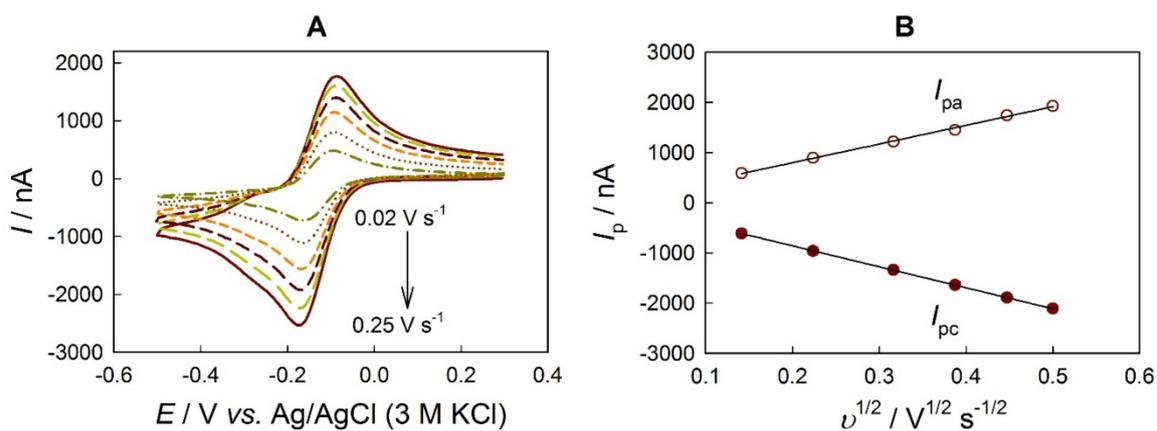
**Figure S5.** (A) CV curves recorded at different  $v$ , and (B) the corresponding plot of the peak currents versus  $v^{1/2}$  for a probe DNA-modified gold electrode. Measurements were performed in 10 mM Tris buffer (pH 7.4) containing  $200 \mu\text{M RuHex}^{3+}$ .
