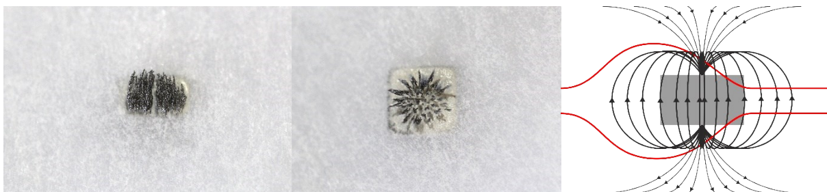
Figure S8: Images of ferrum powder with underlying magnet, top view as presented in the channel ( left ) and side view perpendicular to the channel ( middle ). right: Scheme of the magnet (grey, top view) with channel (red) and magnetic field lines (black).
