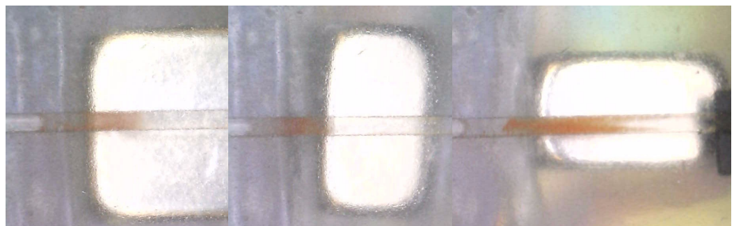
Figure S7: Pictures of three microfluidic channels loaded with the same amount of magnetic beads with same flow velocity, captured on a 5 \times 5 \times 3 mm magnet in three different orientations. (Top view, flow from left to right)
