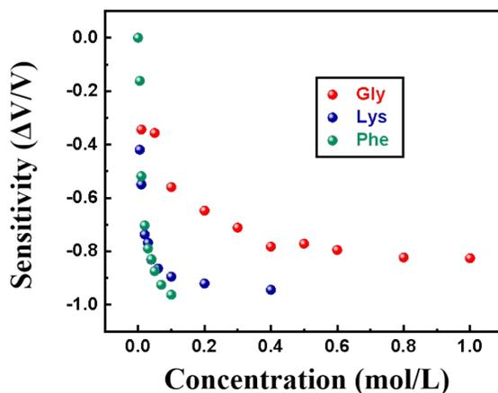
**Figure S5.** The sensitivity result of the TE-based liquid sensor to three amino acids
