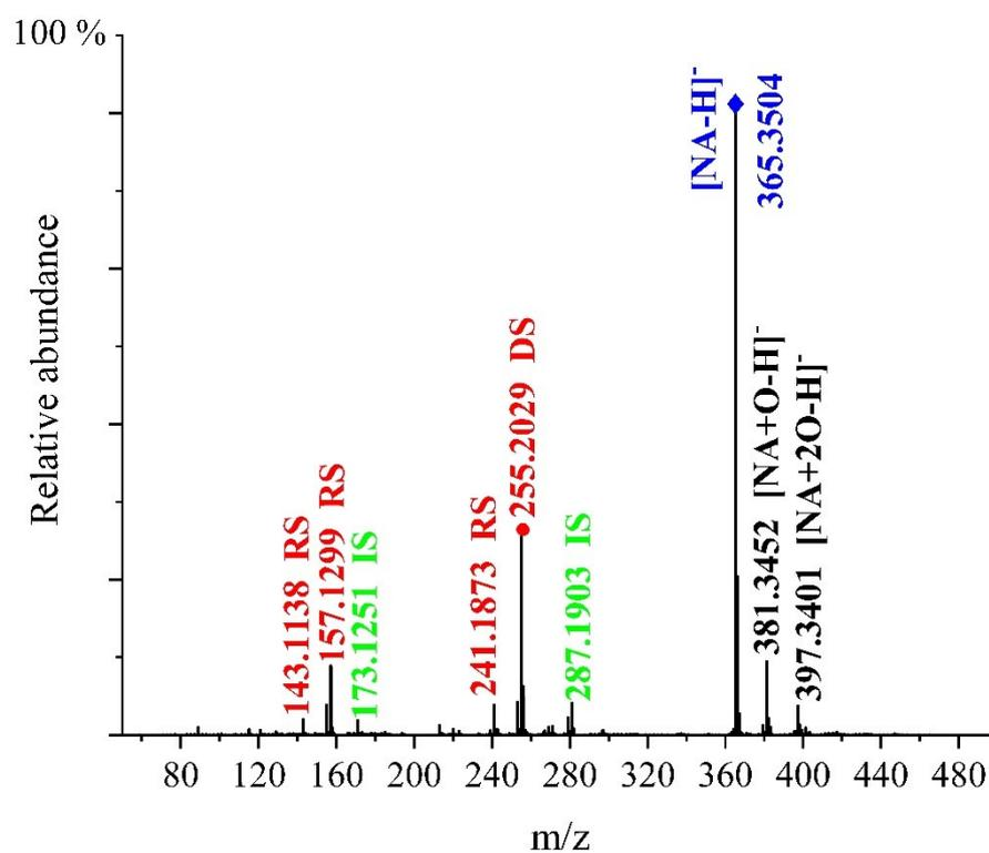
**Figure S4.** Elucidation the location of C=C in NA (24:1(15Z)). Mass spectrum of NA-HAuCl<sub>4</sub> obtained in microdroplet mass spectrometry with a flight distance of 20 mm.
