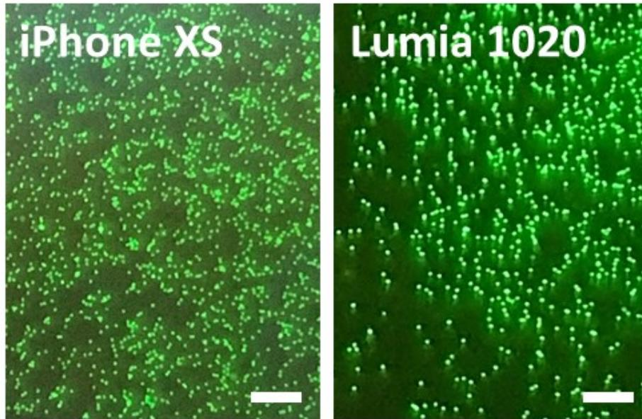
Figure S4. Green fluorescent beads imaged using the SBFM along with an iPhone XS and Nokia Lumia 1020 (Scale bar = 100 $\mu$ m).
