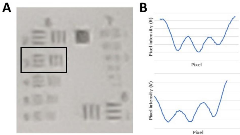
Figure S5: 1951 USAF resolution test chart imaged using S9+ and lens B (10 mm focal length).
