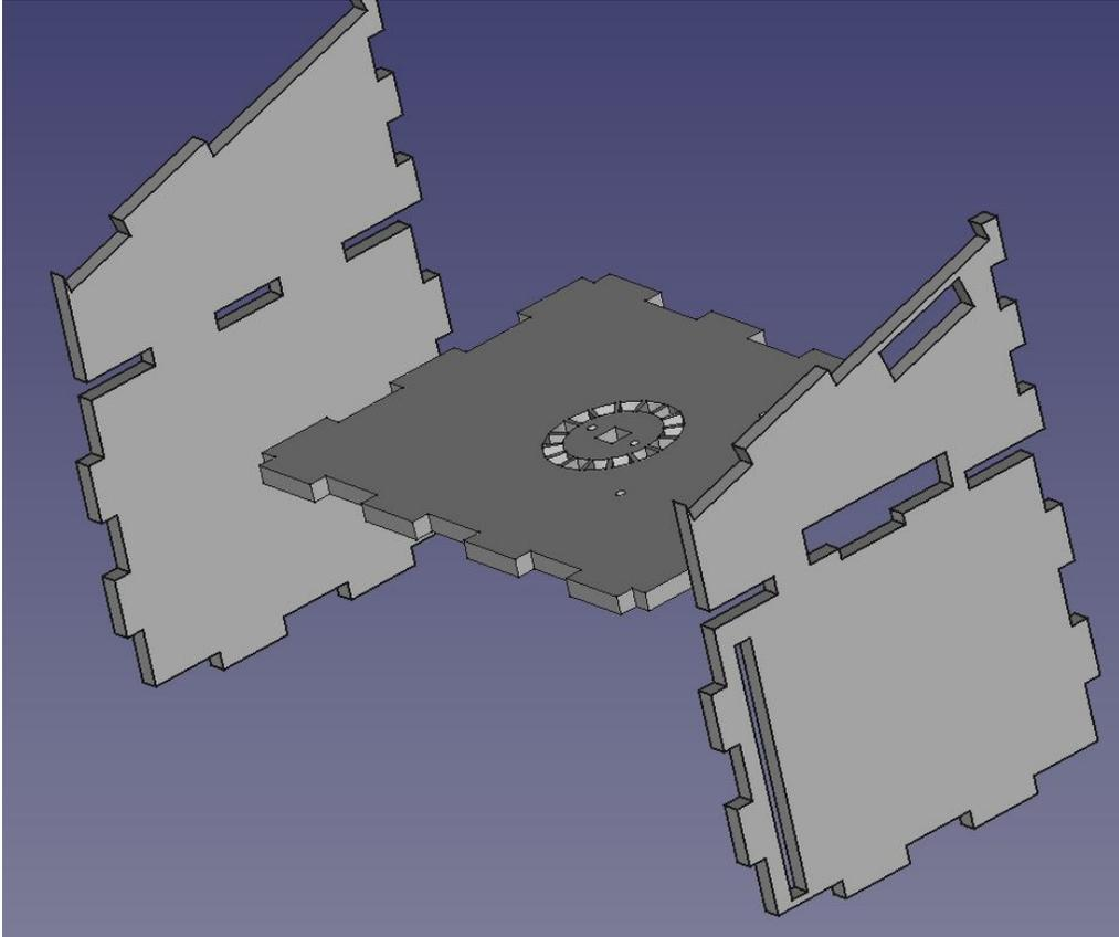
12) Hot glue the [BOTTOM\_REAR] and [BOTTOM\_FRONT] plates so that the holes in the [BOTTOM\_REAR] plate align with the raspberry pi.
