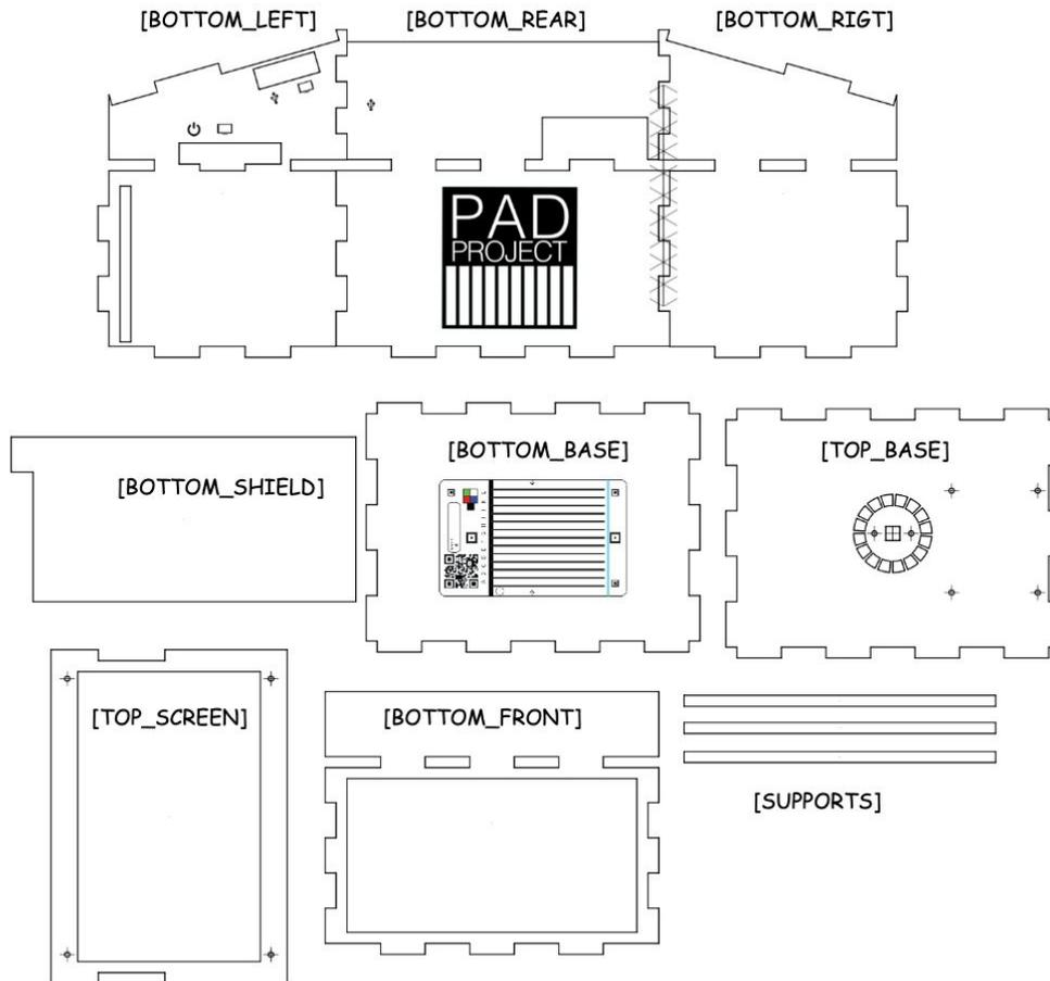
**Fig 2. Diagram of plywood casing pieces**
