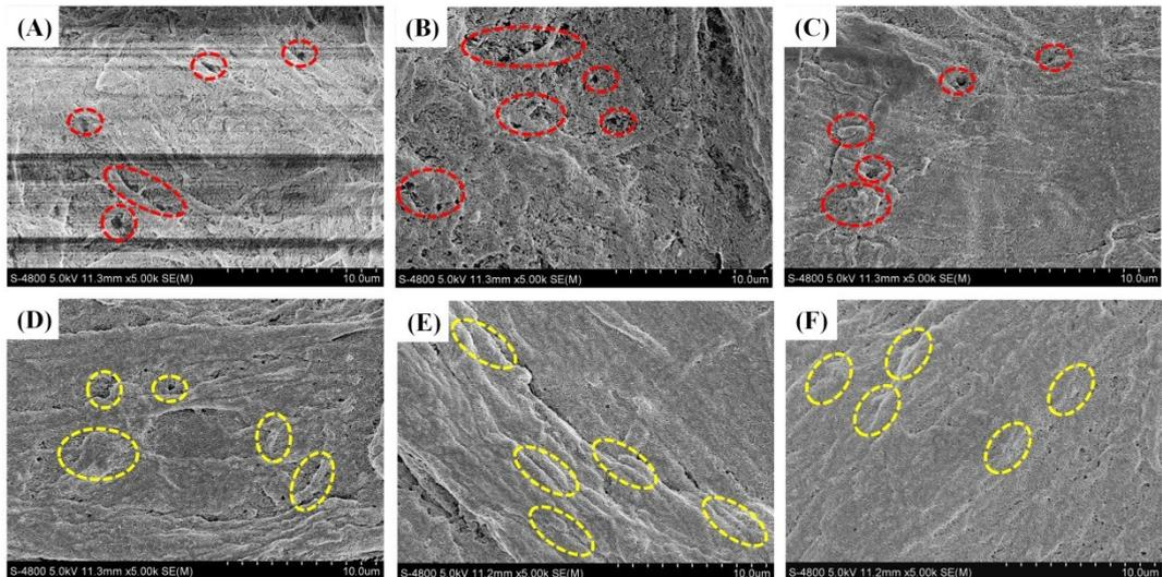
Fig. S5 SEM images of Au@Ag NRs self-assembly monolayer deposited on filter paper with various layers from 1 to 6 at low magnification (A)~(F).
