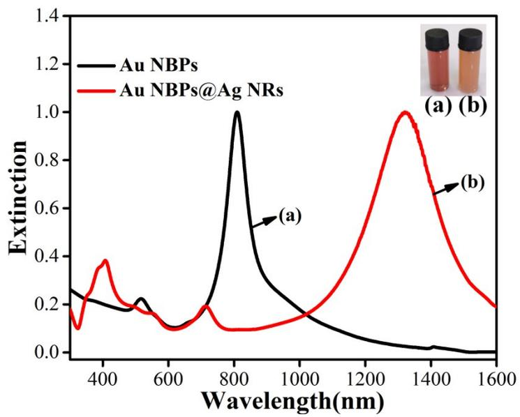
**Fig. S2** Extinction spectrum of Au NBPs and Au@Ag NRs, inset: the photograph of Au NBP colloid and Au@Ag NRs colloid.
