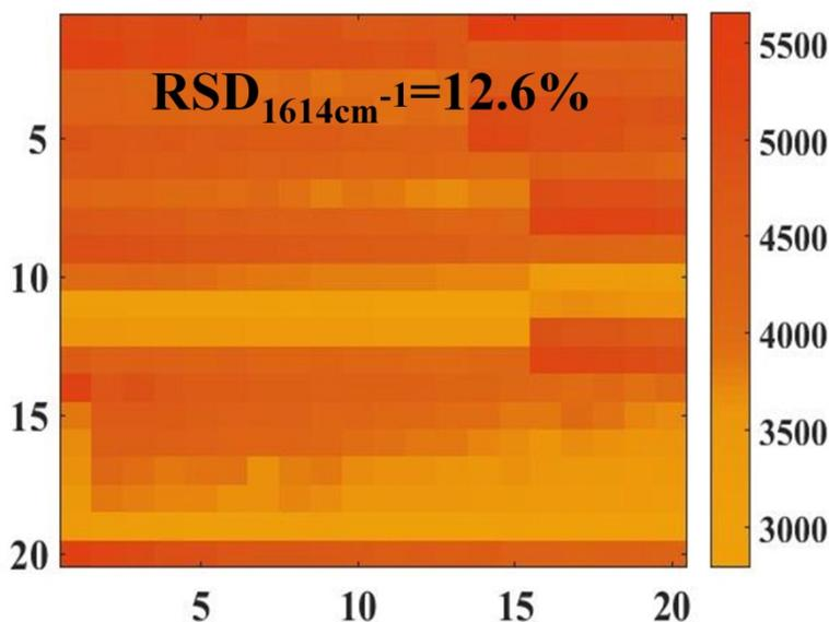
**Fig. S8** SERS spectra of CV ( $10^{-5}$  M) aqueous solution based on paper-based sensor of 400 different points using the Au@Ag NRs monolayer deposited on filter paper. The laser power is 15% and the integration time is 10 s.
