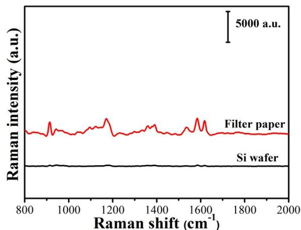
**Fig. S6** Normal Raman spectra of CV based on blank Si wafer and filter paper. The laser power is 15% and the integration time is 10 s.
