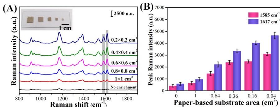
**Fig. S9** (A) SERS spectra of CV with concentration of  $10^{-5}$  M based on paper-based PDMS-assisted platform with various areas; (B) The corresponding SERS intensity of CV with concentration of  $10^{-5}$  M based on paper-based PDMS-assisted platform with various areas.
