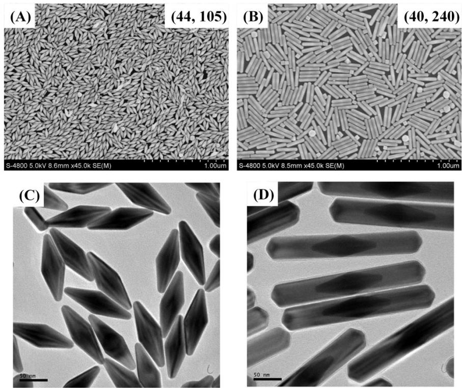
**Fig. S1** (A) SEM image of Au NBPs; (B) SEM image of Au@Ag NRs; (C) TEM image of Au NBPs; (D) TEM image of Au@Ag NRs.
