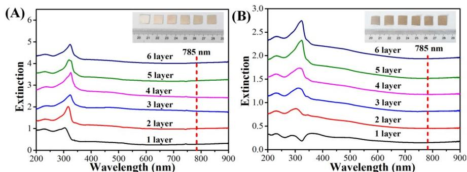
**Fig. S7** The extinction spectra of the SERS substrates deposited on Si wafers (A) and filter paper (B) with different layers. Inset: the corresponding photography of Si wafer-based substrate and paper-based substrate with different layers of nanorods.
