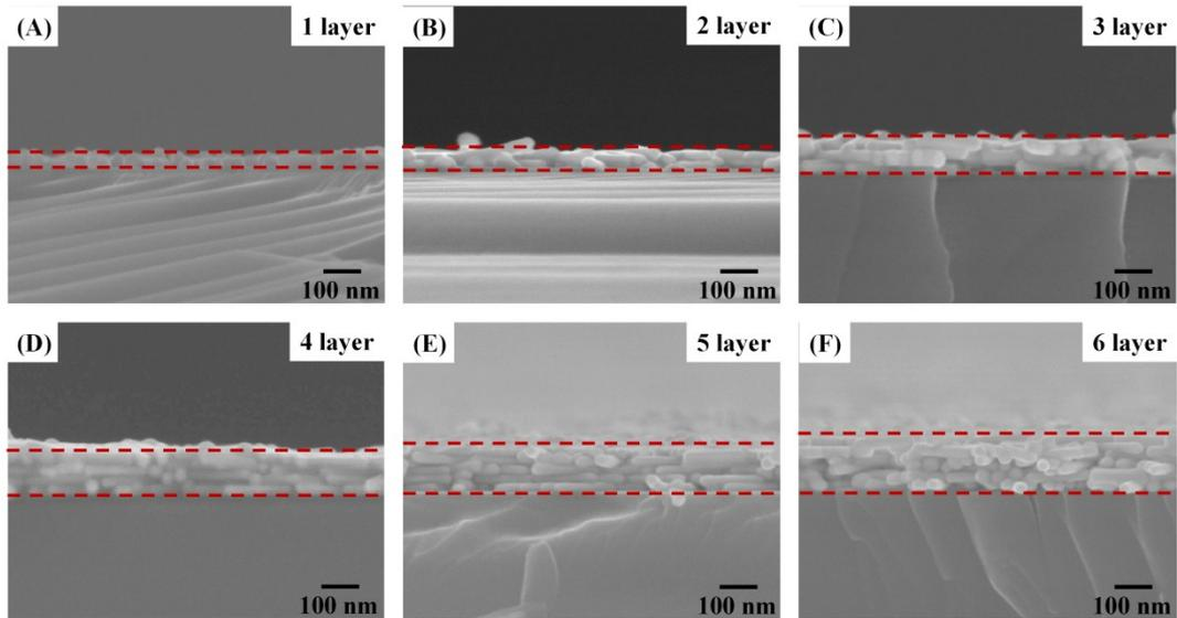
Fig. S4 Cross sectional SEM images of Au@Ag NRs self-assembly monolayer deposited on Si wafer with various layers from 1 to 6 in sectional view (A)~(F).
