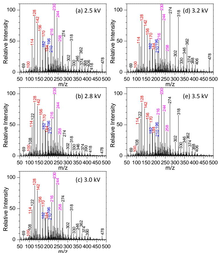
**Figure S1.** Effect of spray voltage on the performance of gasoline analysis: (a) 2.5 kV; (b) 2.8 kV, (c) 3.0 kV, (d) 3.2 kV, and (e) 3.5 kV (Note: applied voltage: 3.5 kV; sample volume: 25  $\mu$ L; percentage of gasoline in methanol: 70%).
