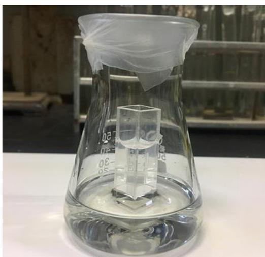
**Figure S10.** Device-2 for FA gas detection by **ZIF-90-LW** suspension
