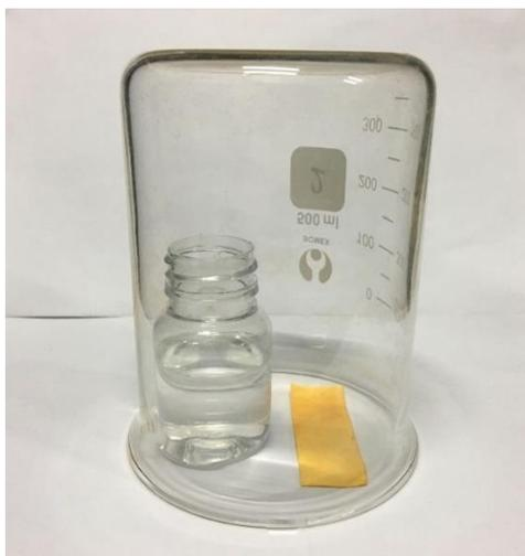
**Figure S9.** Device-1 for FA gas detection by **ZIF-90-LW** test paper.
