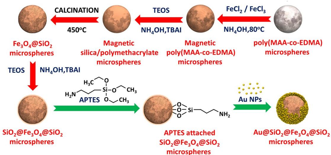
**Figure S1.** The schematical representation of the synthesis protocol for Au@SiO<sub>2</sub>@Fe<sub>3</sub>O<sub>4</sub>@SiO<sub>2</sub> microspheres.
