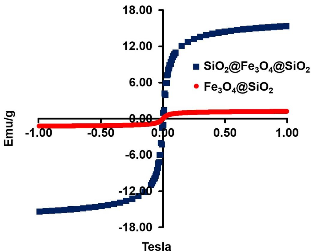
**Figure S2.** Magnetization curves of Fe<sub>3</sub>O<sub>4</sub>@SiO<sub>2</sub> and SiO<sub>2</sub>@Fe<sub>3</sub>O<sub>4</sub>@SiO<sub>2</sub> microspheres obtained by vibrational sample magnetometry after acid leaching. Amount of microspheres: 100 mg, HCl solution (5 % w/w): 25 mL. Shaking rate: 120 cpm, Temperature: 80°C, Time: 6 h.
