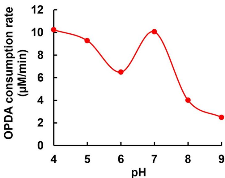
**Figure S3.** The variation of peroxidase like activity with pH for Au@SiO<sub>2</sub>@Fe<sub>3</sub>O<sub>4</sub>@SiO<sub>2</sub> microspheres. Reaction volume: 4 mL, Microsphere amount: 10 mg, pH 7.0, H<sub>2</sub>O<sub>2</sub> solution: 2 µL, OPDA concentration: 400 µM, Rotating rate: 120 cpm, Room temperature, 90 min.
