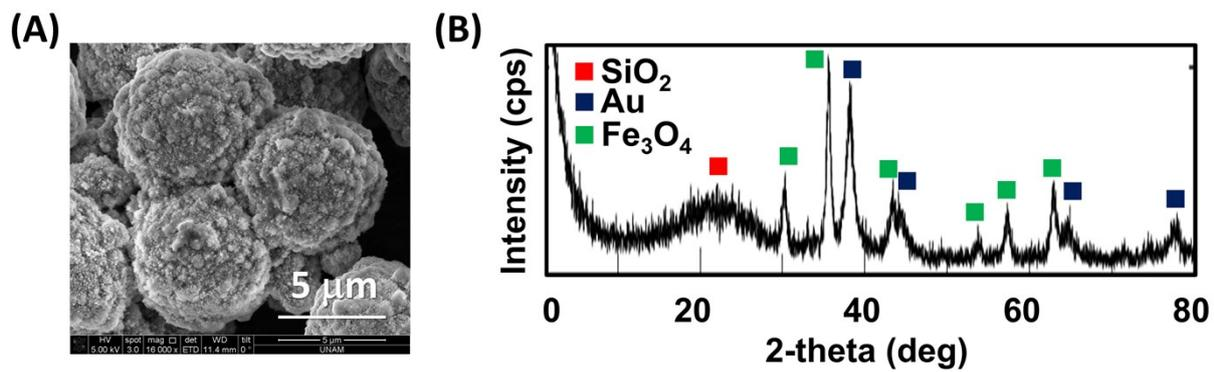
**Figure S5.** (A) SEM image, and (B) XRD spectrum of Au@SiO<sub>2</sub>@Fe<sub>3</sub>O<sub>4</sub>@SiO<sub>2</sub> microspheres after colorimetric determination of GSH via peroxidase-like reaction.
