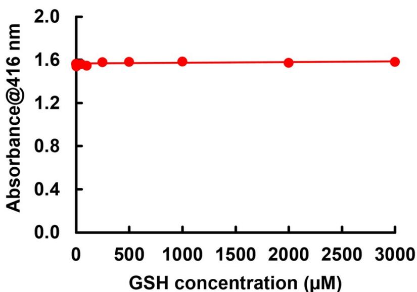
**Figure S4.** The effect of added GSH concentration on the resulting absorbance obtained by the colorimetric conversion in the absence of GSH. Concentration of Au@SiO<sub>2</sub>@Fe<sub>3</sub>O<sub>4</sub>@SiO<sub>2</sub> microspheres: 2.5 mg/mL, H<sub>2</sub>O<sub>2</sub>: 2 µL, Initial OPDA concentration: 400 µM, Time: 30 min, Rotating rate: 100 cpm, Room temperature.
