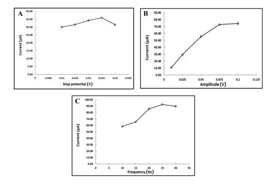
**Fig. S5.** Optimization of square wave voltammetric parameters for histamine detection using unmodified SPGE: (A) step potential, (B) amplitude, and (C) frequency
