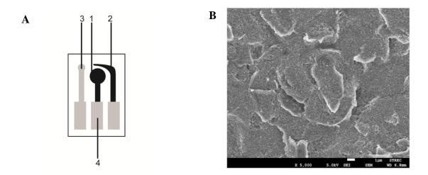
**Fig. S1.** (A) Screen-printed graphene electrode (SPGE). Graphene ink was printed to obtain the working electrode (1) and auxiliary (2), respectively. Ag/AgCl ink was printed to obtain the reference electrode (3) and conducting pads or electric contacts (4). (B) SEM images of surface morphology of graphene screen-printed electrodes.
