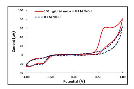
**Fig. S3.** Cyclic voltammograms obtained from unmodified SPGE in 0.2 M NaOH (blue line) and 100 mg/L histamine in 0.2 M NaOH (red line), respectively.
