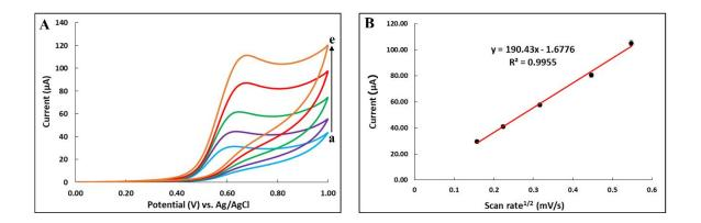
**Fig. S4.** (A) Cyclic voltammograms of histamine at unmodified SPGE in 0.2 M NaOH using different scan rates (a-e: 25, 50, 100, 200, and 300 mV/s, respectively), (B) Plot of the anodic peak currents *versus* the square root of the scan rate.
