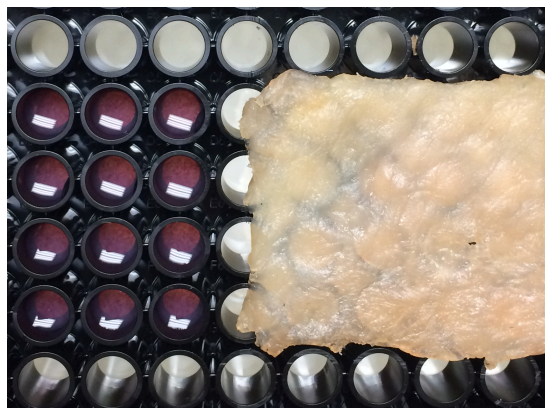
Figure S2. Digital photograph of experimental set-up for Au-polyester NP synthesis by irradiation through chicken tissue barrier.
