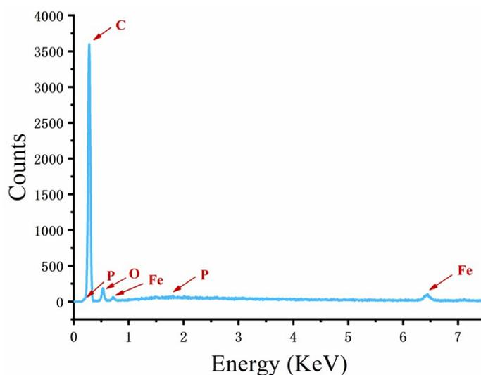
**Fig. S2** The characterization of SEM-EDX spot analysis of P-Mag-LPNs. The characteristic EDX spectrum of P-Mag-LPNs validates the existence of Fe and P elements.
