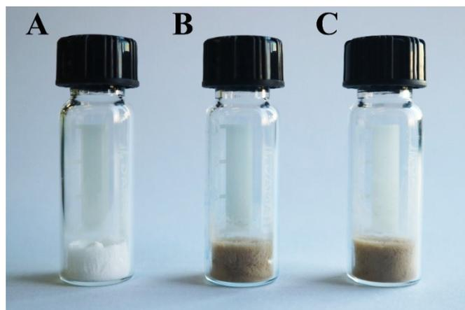
**Fig. S1** Appearance of lyophilized powder of lipid-polymer hybrid ultrasound contrast agents. (A) Appearance of lyophilized powder of LPNs. (B) Appearance of lyophilized powder of Mag-LPNs. (C) Appearance of lyophilized powder of P-Mag-LPNs. The lyophilized powder of Mag-LPNs exhibit brownish color as compared to LPNs exhibiting white color. But there are no obvious differences between the appearance or color of Mag-LPNs and P-Mag-LPNs.
