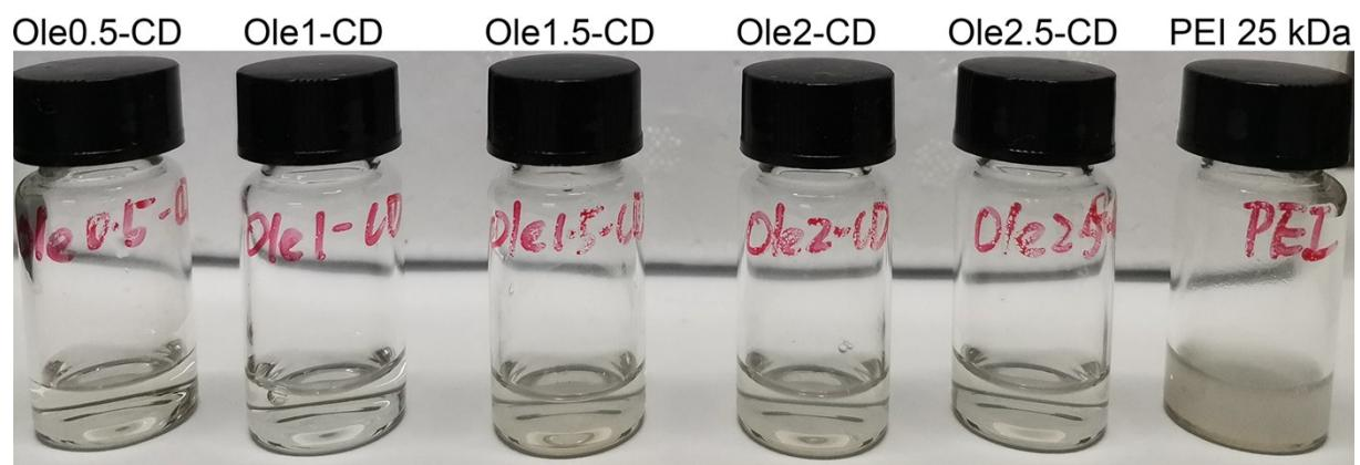
**Fig. S12.** BSA adsorption assays, photographs show the PEI solution(0.5 mg/mL) turned turbid by addition of BSA(1mg/mL), while Ole-CD solution(0.5 mg/mL) is still clear.
