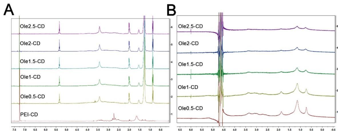
**Fig. S3.** <sup>1</sup>H NMR spectrum of PEI-CD and Ole-CDs in CDCl<sub>3</sub>(A) and D<sub>2</sub>O (B).
