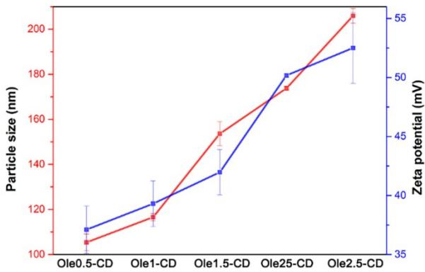
**Fig. S6.** Mean DLS particle sizes (red) and surface charge (blue) of **Ole-CDs** under the concentration of 20 mg/L. Data represent mean  $\pm$  SD ( $n = 3$ ).
