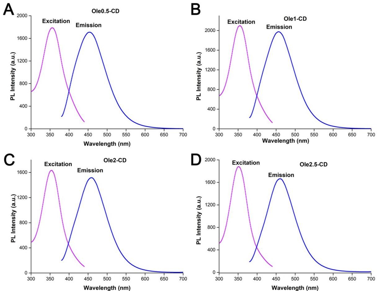
**Fig. S8.** The maximum PL excitation and emission spectra of **Ole-CDs** aqueous solution, (A) **Ole0.5-CD**, (B) **Ole1-CD**, (C) **Ole2-CD**, (D) **Ole2.5-CD**.
