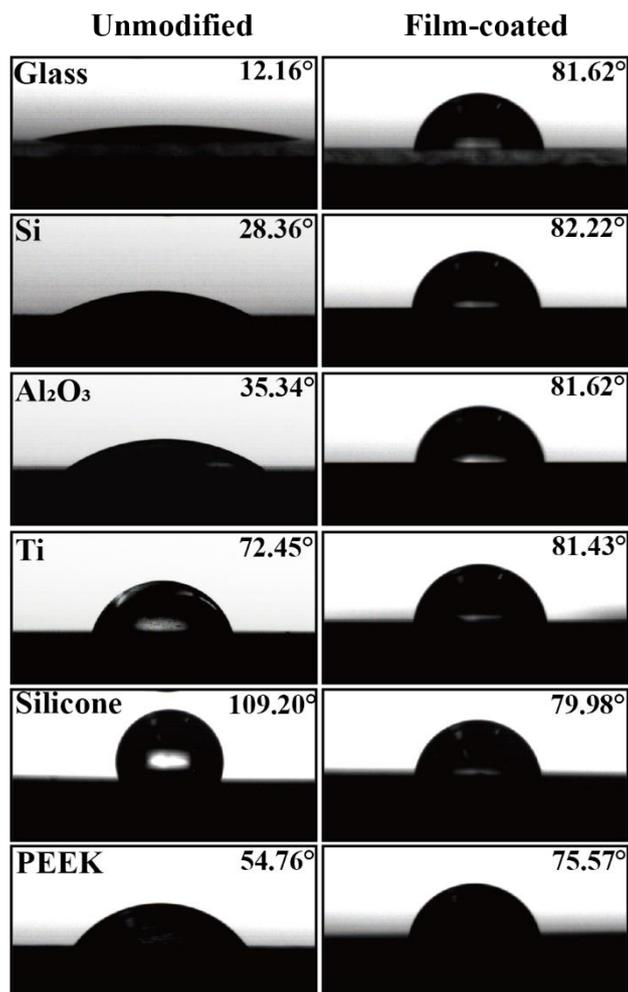
Figure S4. Images of water contact angle on the substrate before (left) and after (right) PTB@ $\epsilon$ -PL coating. The reaction time was 120 min, and the phase transition solution was prepared as follows: BSA ( $10 \text{ mg mL}^{-1}$  in water), TCEP ( $50 \text{ mM}$ , pH 4.5 in water) and  $\epsilon$ -PL ( $0.4 \text{ g mL}^{-1}$  in water) were mixed in a volume ratio of 1: 1: 1.
