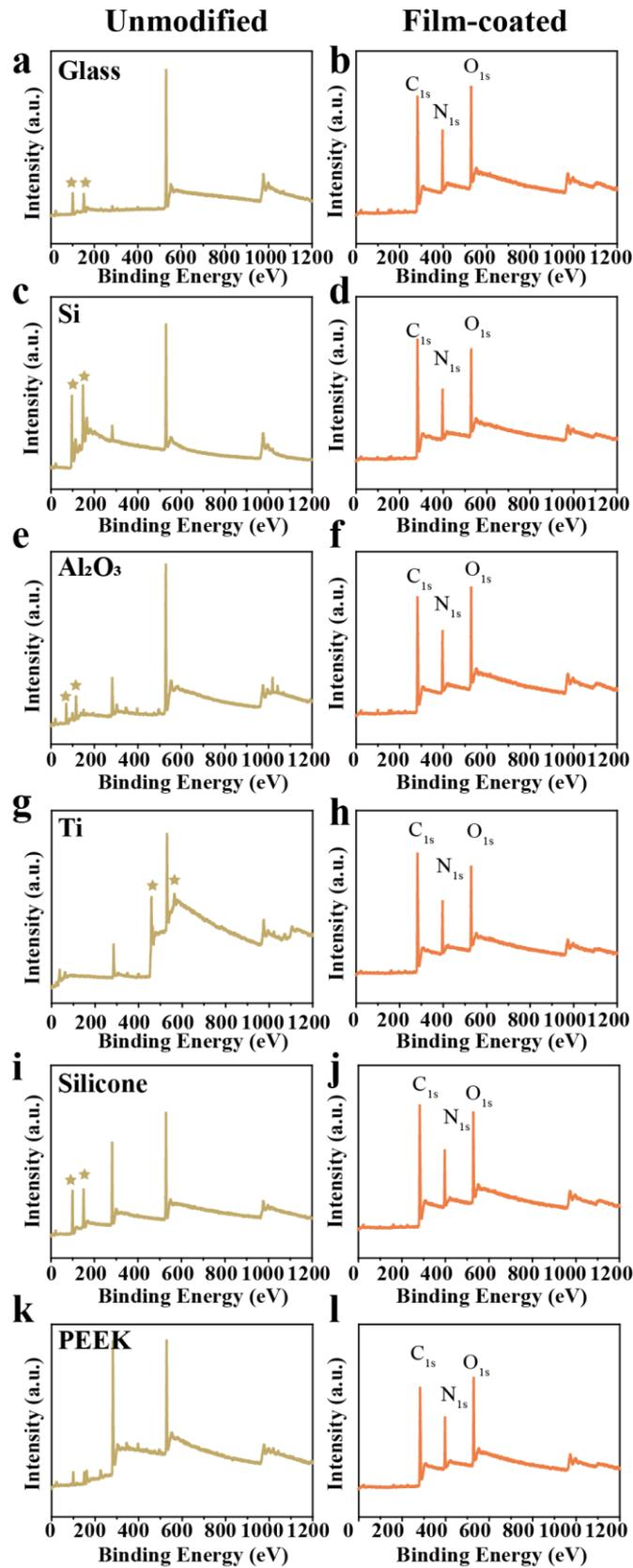
Figure S5. XPS characteristic of the PTB@ $\epsilon$ -PL nanofilm adhered onto various substrates. (a, c, e, g, i, k) XPS wide scan of bare substrates. (b, d, f, h, j, l) XPS wide scan of various substrates with the coating of the nanofilm.
