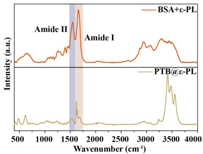
Figure S2. The comparison of the FTIR peaks between the PTB@ε-PL nanofilm and the mixture of native BSA and ε-PL.
