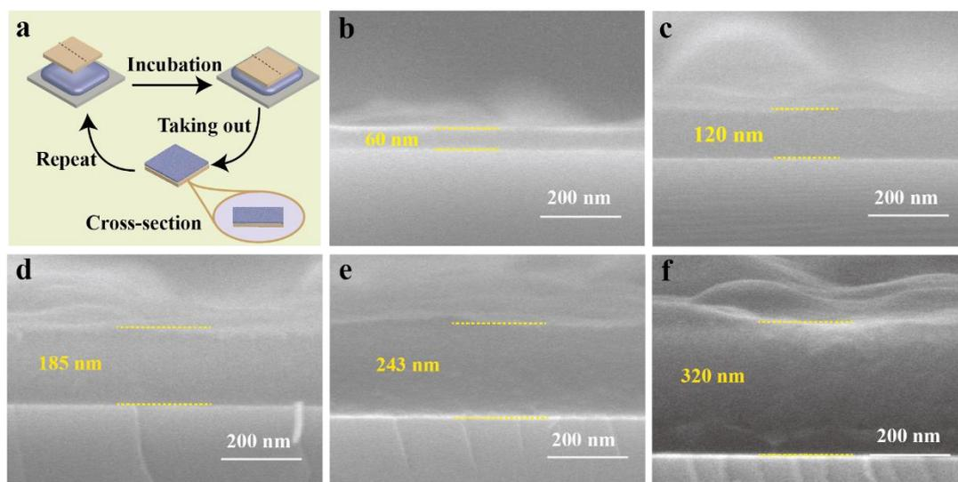
Figure S7. Cross-section SEM images of the PTB@ $\epsilon$ -PL nanofilm coated on Si with different coating time. (a) Schematic cartoon showing the method of preparing multilayer coating. (b-f) The cross-sectional SEM images after preparing the 1-5 layers of the PTB@ $\epsilon$ -PL coating on Si. The dotted line representing the upper and lower edges of the coating in cross-sectional view.
