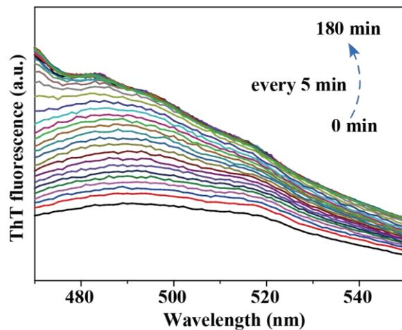
Figure S3. The ThT fluorescence spectra of the PTB@ $\epsilon$ -PL samples with different reaction time. The arrow indicating the intensity enhancement with increasing the reaction time from the bottom curve to the top curve, at a time interval of 5 min within 180 min.
