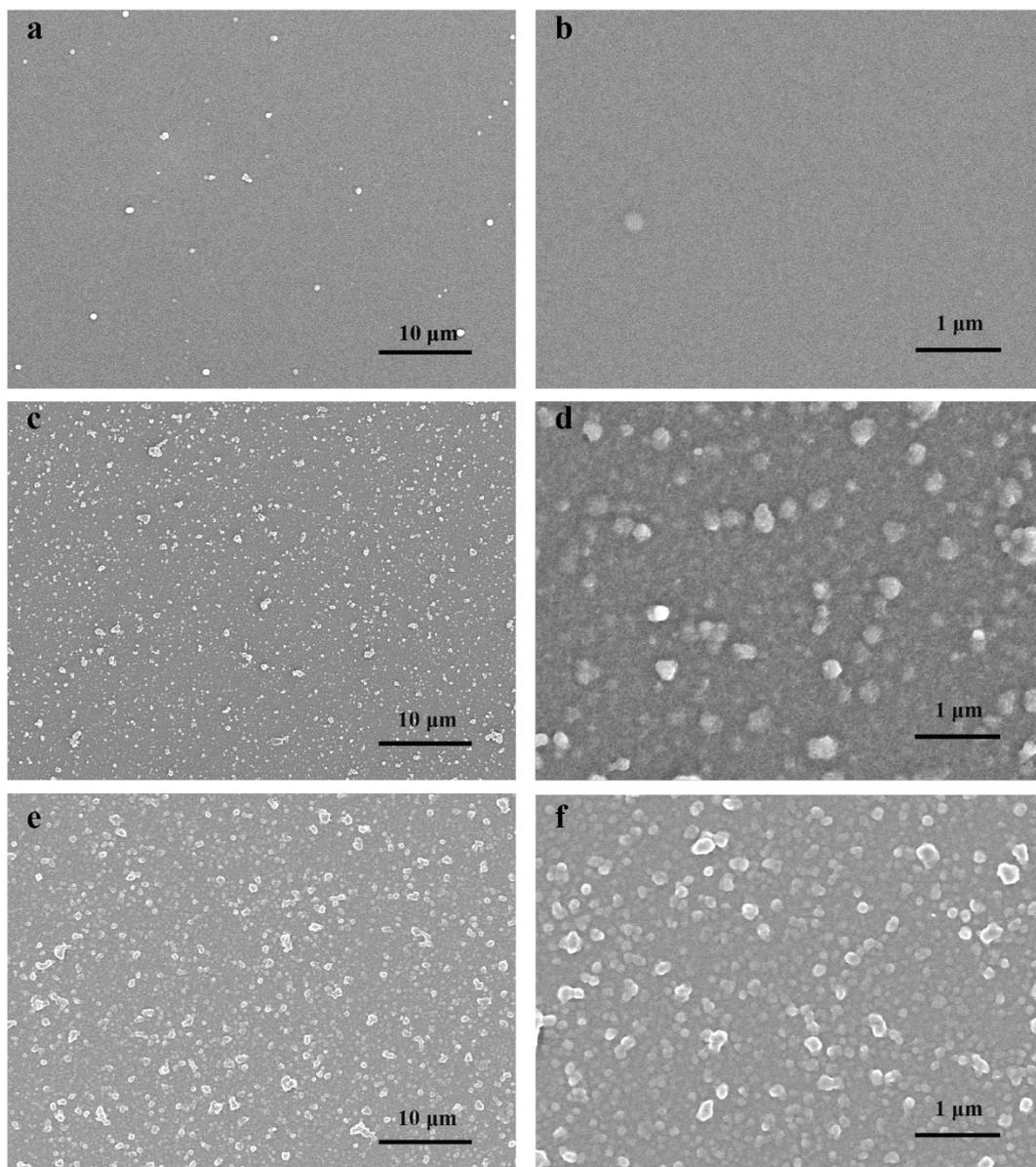
Figure S13. SEM images showing the surface morphology of PTB@ $\epsilon$ -PL coating at different BSA concentration in the phase transition solution. (a, b) BSA 5 mg mL<sup>-1</sup>, (c, d) BSA 10 mg mL<sup>-1</sup>, (e, f) BSA 20 mg mL<sup>-1</sup>. The reaction time is 2 h, and the phase transition solution was prepared by mixing BSA aqueous solution, TCEP (50 mM, pH 4.5 in water) and  $\epsilon$ -PL (0.4 g mL<sup>-1</sup> in water) in a volume ratio of 1: 1: 1.
