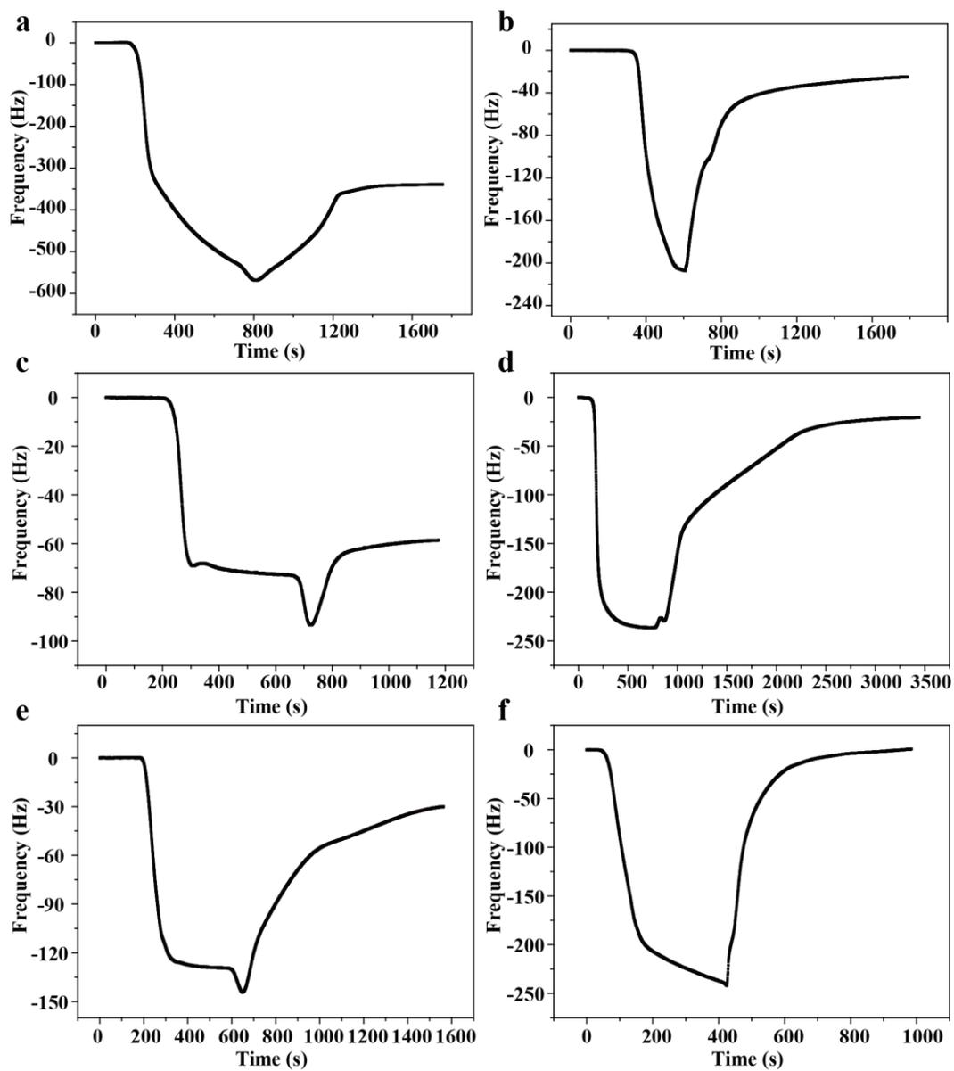
Figure S16. QCM frequency shift as function of time during the adsorption of human serum (a, b), FBS (c, d), and bacterial lysate (e, f) on bare Au chips (a, c, e) or the PTB@ $\epsilon$ -PL-coated Au chip (b, d, f).
