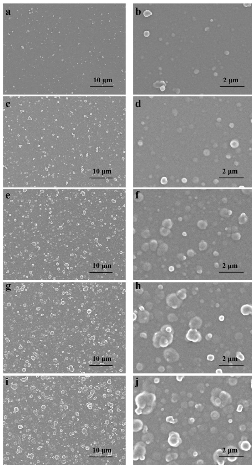
Figure S15. SEM images showing the surface morphology of 1 (a, b), 2 (c, d), 3 (e, f), 4 (g, h) and 5 (i, j) layers of PTB@ $\epsilon$ -PL coating. The reaction time is 2 h, and the phase transition solution was prepared by mixing BSA aqueous solution ( $10 \text{ mg mL}^{-1}$ ), TCEP (50 mM, pH 4.5 in water) and  $\epsilon$ -PL ( $0.4 \text{ g mL}^{-1}$  in water) in a volume ratio of 1: 1: 1.
