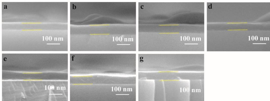
Figure S17. Cross-section SEM images of the PTB@ $\epsilon$ -PL nanofilm coated on silicon wafer before (a) and after challenged by ultrasound (b), 3M adhesive tape peeling (c), autoclaving (d), DMSO (e), artificial saliva (f) and artificial urine (g). The dotted line representing the upper and lower edges of the coating in cross-sectional view.
