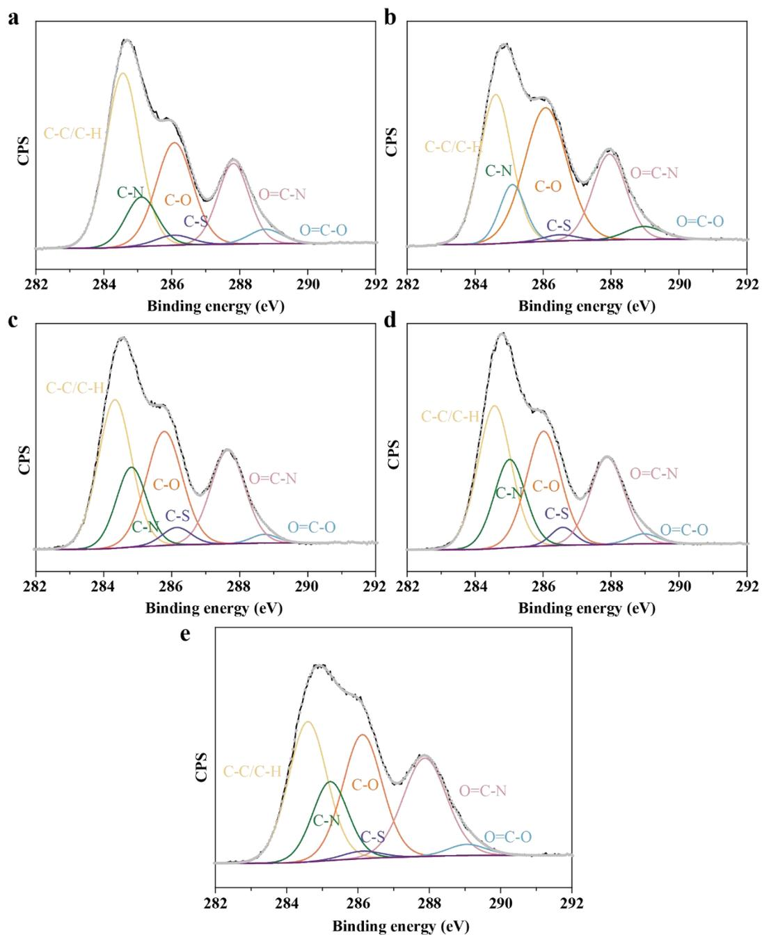
Figure S8. High-resolution C1s deconvolution spectra of 1 (a), 2 (b), 3 (c), 4(d) and 5 layers PTB@ε-PL coating on Si.
