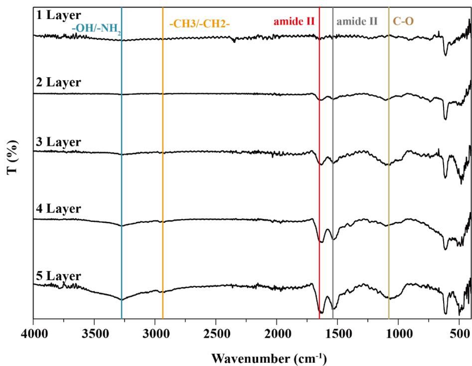
Figure S9. ATR- FTIR spectra of 1-5 layers PTB@ $\epsilon$ -PL coating on Si.
