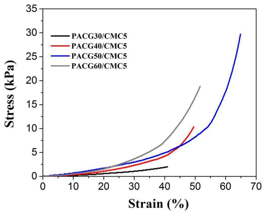
**Figure S6.** Compression stress-strain curves of PACG/CMC sponges with various ACG contents from 30% to 60% after absorbing water.
