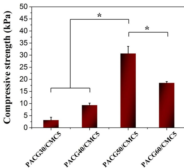
**Figure S7.** Compressive strength of PACG/CMC sponges with various ACG contents after absorbing water. Error bar indicates S.D. (n=3)
