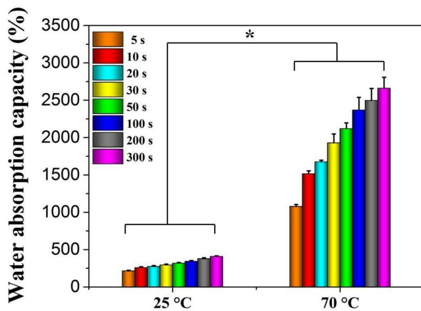
**Figure S4.** Water absorption capacity of PACG50/CMC5 sponges gelled at 25 °C and 70 °C at different times. Error bar stands for S.D. (n=3)
