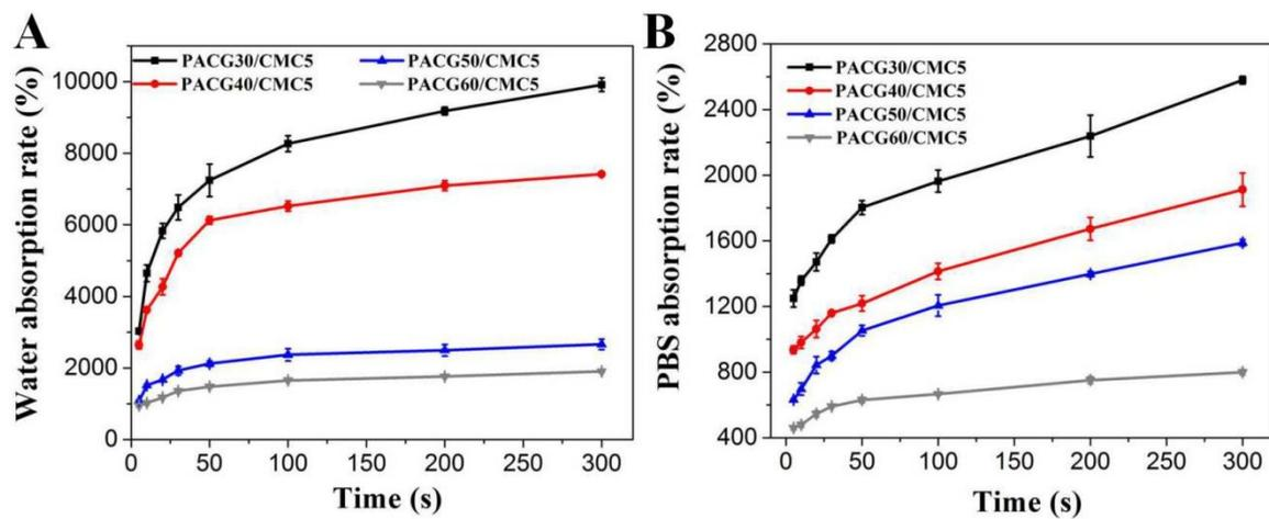
**Figure S5.** Water (A) and PBS (B) absorption rates of PACG/CMC sponges with various ACG contents from 30% to 60%. Error bar indicates S.D. (n=3)
